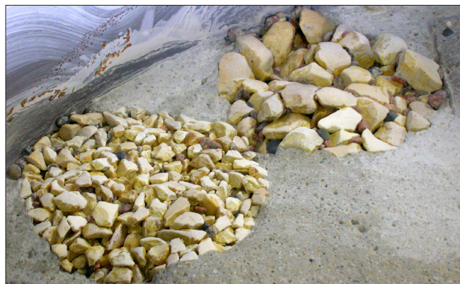
Figure 15 Abrasive test results of PUR-stone specimens made of 8/11 mm limestone and 16/32 mm limestone
