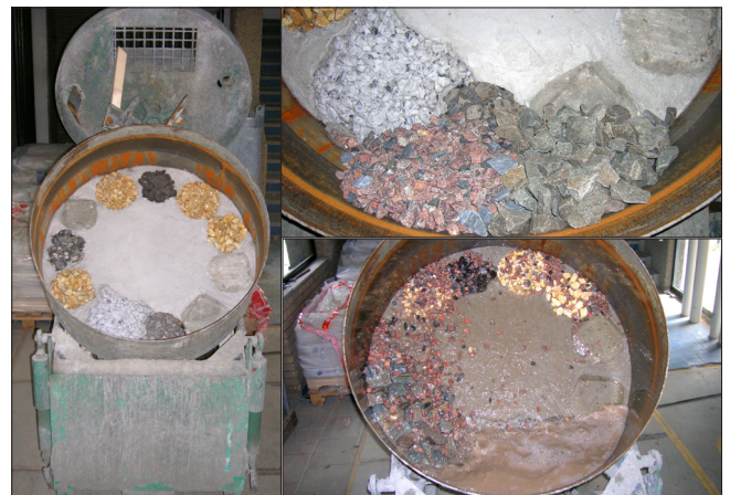
Figure 13 Set-up of relative resistance to abrasive action test
