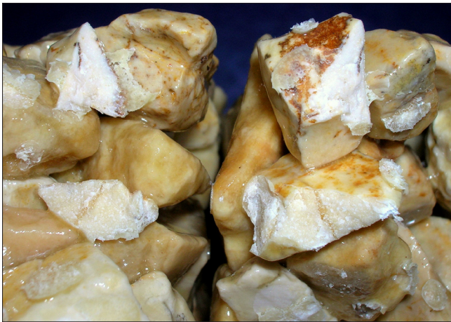
Figure 5 Broken stones at the broken cross section of yellow beam 6 in the monotonic three-point bending strength test
