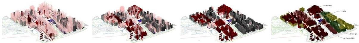
Fig. 2: Retrofit steps every 5 years starting from 2017 with building of average heat consumption over 300 kWh/m<sup>2</sup>
