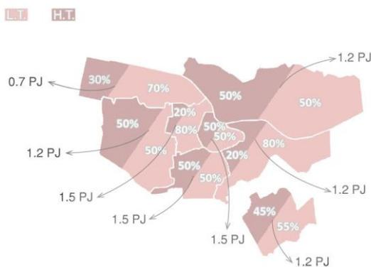
Fig. 3: High Temperature and Low temperature systems ratio per district
