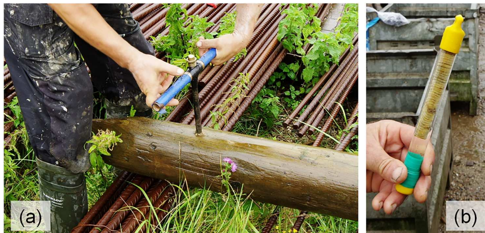
Figure 2. Sample collection: (a) extraction of a drill core from the tip of a retrieved timber foundation pile in Amsterdam, and (b) drill core collected in a plastic tube filled with water.
