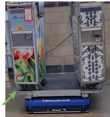
Figure 3.20: The arrow points towards the metal rod used to simulate an elongated AGV clamp. It can be seen that the trolleys do not remain flush to the ULD.
