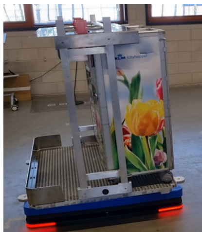
Figure 3.22: During testing no trolleys fell off and the trolleys remained flush to the ULD.
