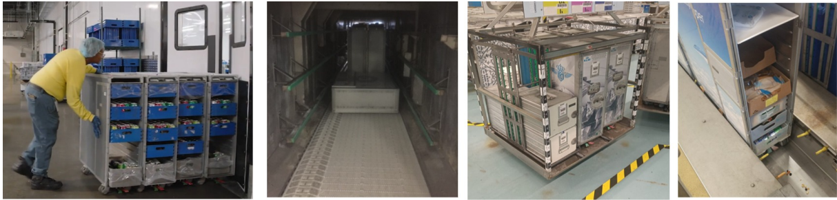
Figure 1: All methods of airline catering trolley transport used inside airline catering facilities, left to right: manual, moving floor conveyor, monorail, side actuated conveyor
