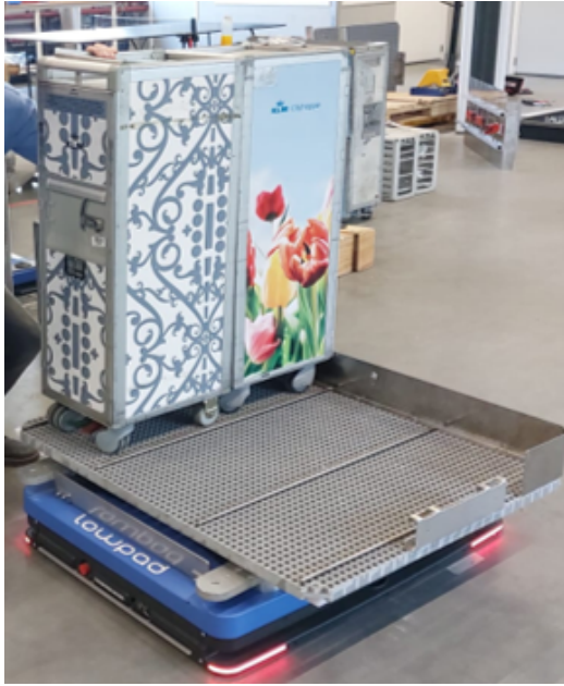
Figure 14: During testing without the sides the trolleys tipped over the sides.
