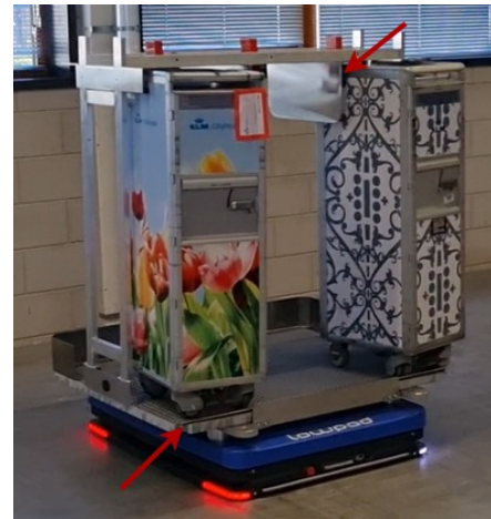
Figure 11: No trolleys fell after increasing the AGV clamp and the Trolley dividers length.
