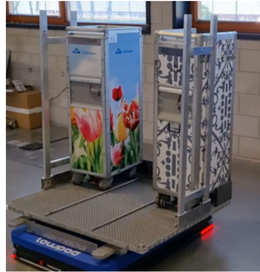
Figure 15: With the added sides, no trolleys fell off during testing and the trolleys remained flush.
