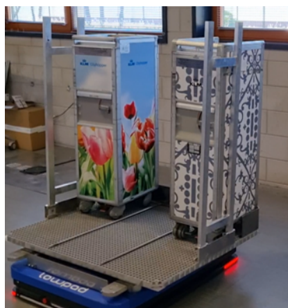
Figure 3.24: With the frame, no trolleys fell of the ULD during testing.
