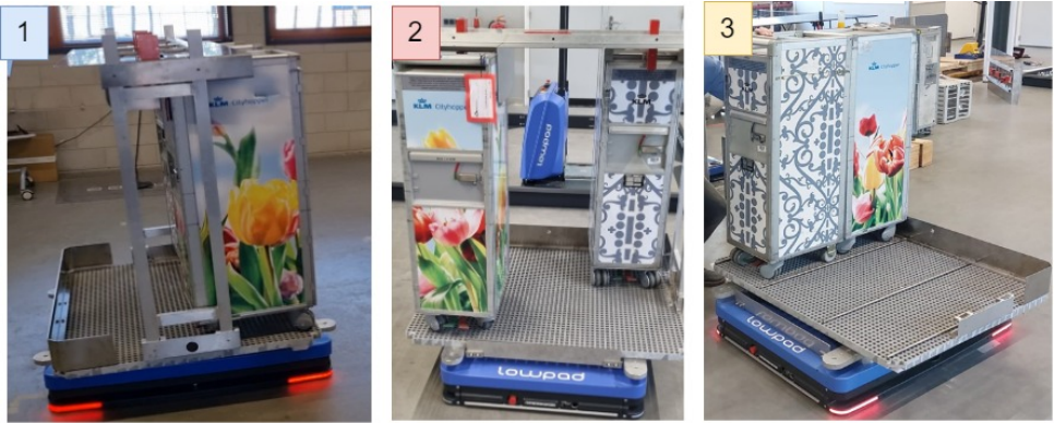
Figure 3.17: The 3 different ULD designs tested at Lowpad. 1 and 3 are inclined, 1 and 2 are usable in a highloader.
