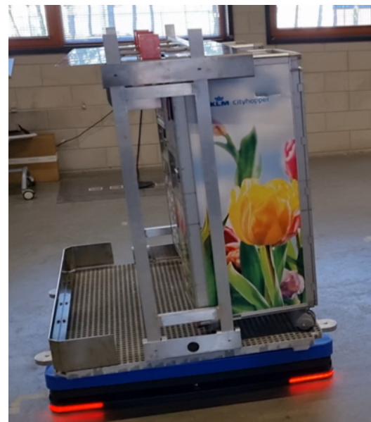
Figure 13: During testing no trolleys fell off and the trolleys remained flush to the ULD.
