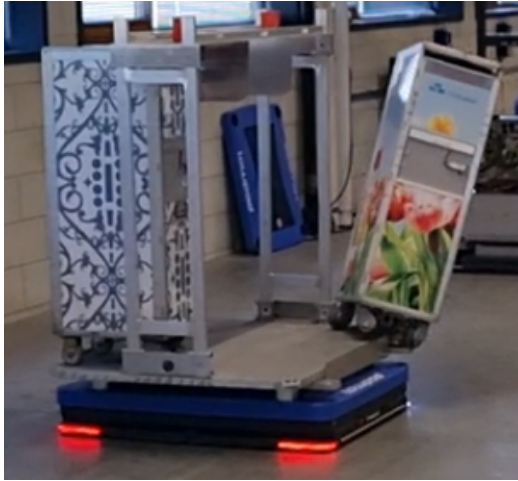
Figure 10: A trolley falling of the ULD during testing.
