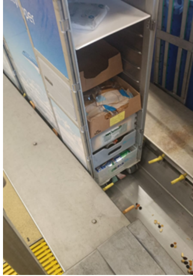
Figure 2.4: A side-gripping conveyor is used to transport all Europa food trolleys past emptying workstations.
