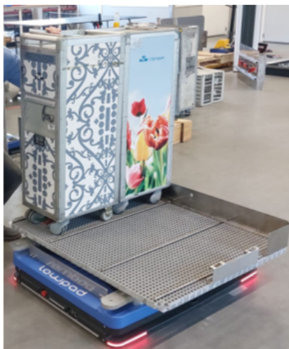
Figure 3.23: During testing without the frame, the trolleys tipped over the sides.
