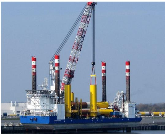
Figure 1.1: A luffing boom crane on a jackup ship.
