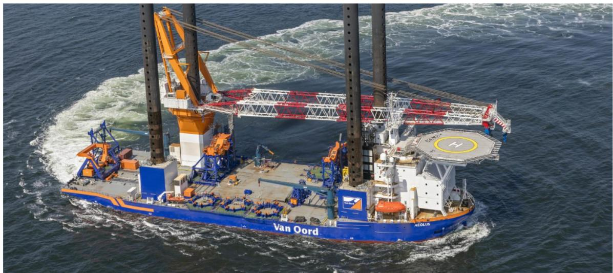
Figure 2.5: Conventional crane on a jackup-ship
