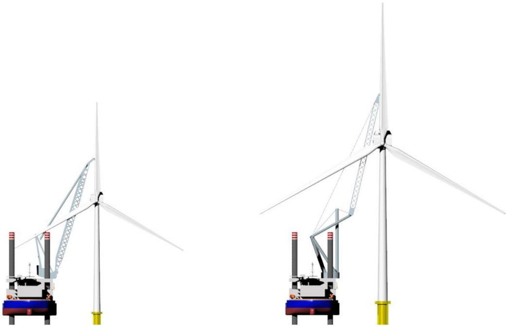
Figure 1.5: Comparison in lifting height of a luffing boom crane (left) and the Tetrahedron crane (right), on the same jackup ship. Clearly, the Tetrahedron crane can install larger wind turbines with the same jackup ship.
