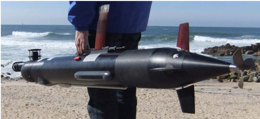
**Figure 1-1:** OceanScan-MST's LAUV [2]
