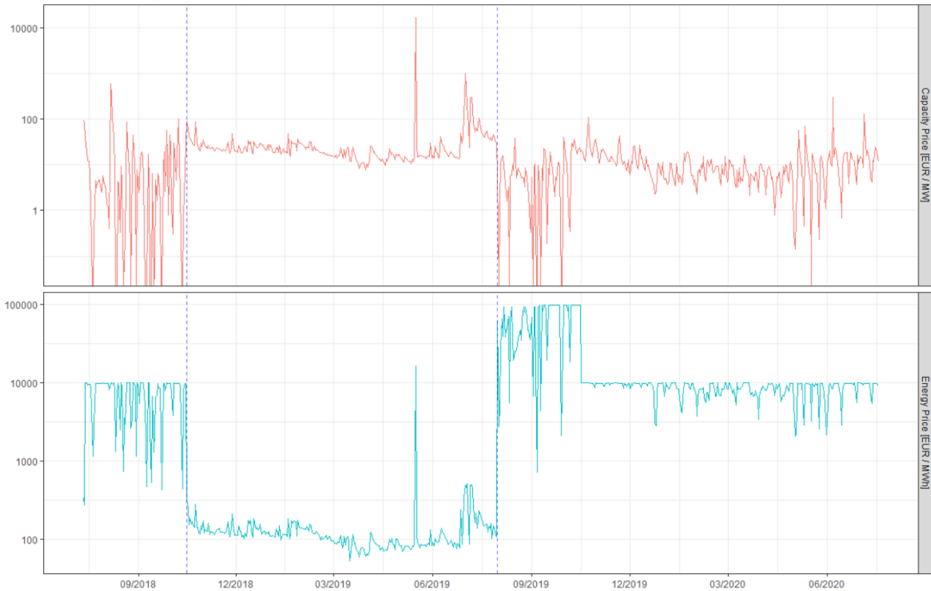
Figure 6.1. The evolution of marginal prices for positive aFRR, balancing capacity (top) and balancing energy (bottom) in Germany from end of 2018 to mid-2020. The period during which 'mixed price calculation' was in force is marked with dashed lines.
