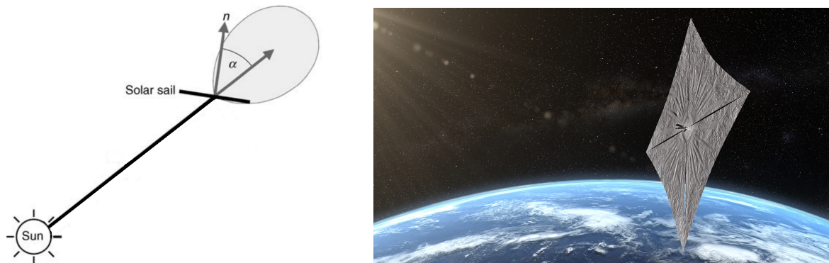
Figure 1.1: (Schematic drawing of solar-sail force bubble (left), edited from [13]. Lightsail-2 artist concept with Earth in the background (right) [14].
