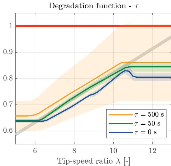
Fig. 4. Varying the wind speed filter time constant to evaluate its effect on the learning performance of the estimated degradation function. It is striking to observe that a perfect (unfiltered,  $\tau = 0$  s) REWS measurement underperforms in terms of the estimated degradation function accuracy to the case when  $\tau = 50$  s. For the severe-filtering case  $\tau = 500$  s, the end-result distribution increases.
