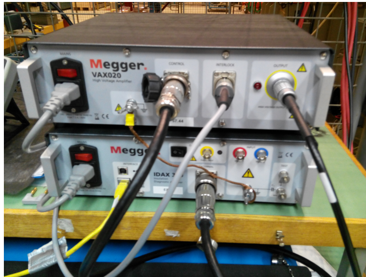
Figure C.1: Megger IDAX 300 and VAX020
