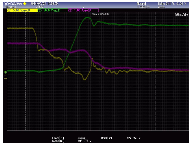
Figure 4.2: Switching of characteristic of an IGBT
