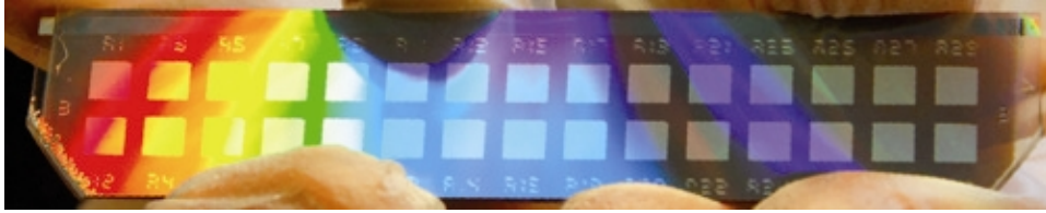
Figure 5.1: Individual solar cells on 3 \times 10 \text{ cm}^2 glass substrate
