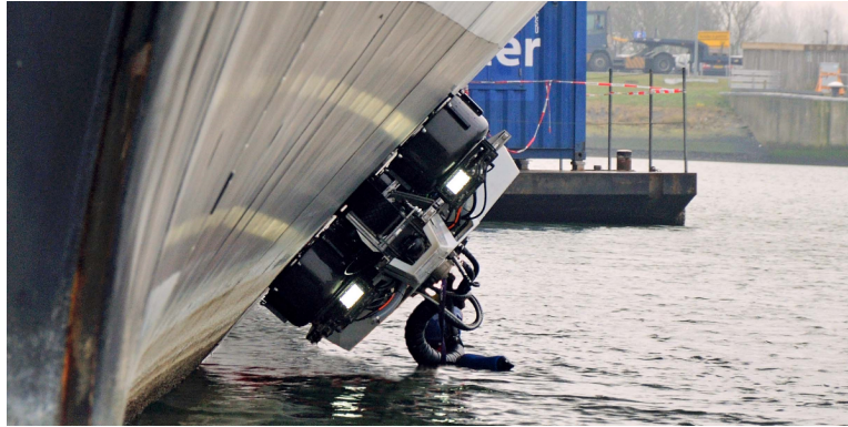
Figure 1-1: The Fleet Cleaner robot attached to a ship's hull.
