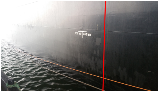
(b) First weld line on the ship.
