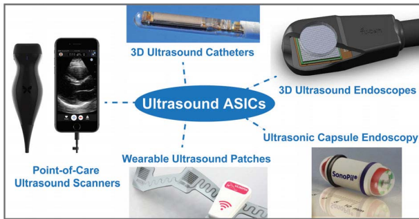
FIGURE 1. Examples of emerging medical ultrasound imaging devices (clockwise from the left): a hand-held point-of-care ultrasound scanner (image courtesy of Butterfly Network) [1]; a 3D intra-cardiac imaging catheter [3]; an artist's impression of a 3D transesophageal ultrasound probe [2]; a pill-shaped ultrasonic endoscopy device (image courtesy of Univ. of Glasgow) [4]; an artist's impression of a wearable ultrasound patch (image courtesy of ULIMPIA project) [6].
