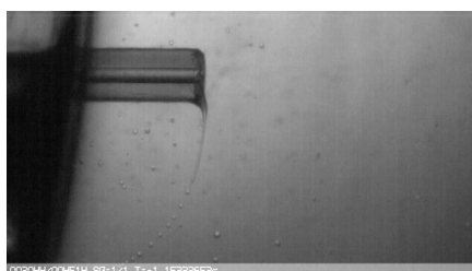
Figure 3.S8: Droplet formation at the capillary orifice at a rotation speed of 2700 rpm. Video recordings of droplet formation at the 100 \mu\text{m} diameter fused silica capillary orifice at a rotation speed of 2700 rpm. The playback speed is 5 fps for a total of 50 frames. [i partial, low-res]
