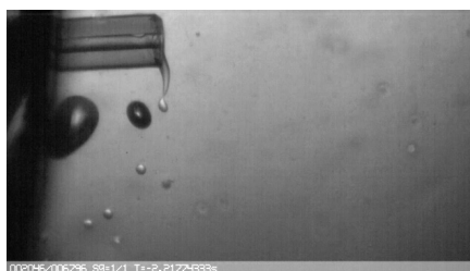
Figure 3.S7: Droplet formation at the capillary orifice at a rotation speed of 1900 rpm. Video recordings of droplet formation at the 100 \mu\text{m} diameter fused silica capillary orifice at a rotation speed of 1900 rpm. The playback speed is 5 fps for a total of 50 frames. [i partial, low-res]
