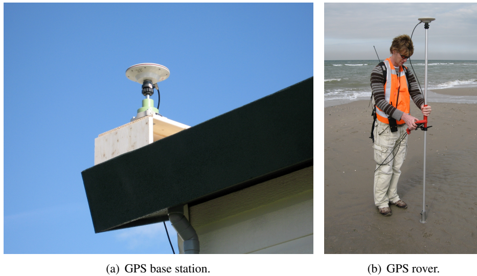
Figure 3.51: GPS base station and rover.
