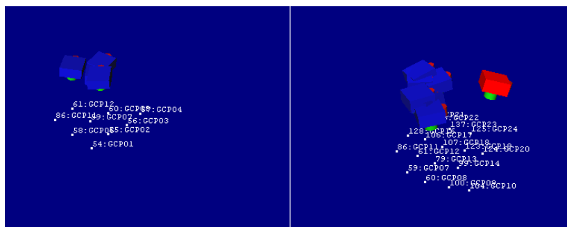
Figure 3.13: The ground control points of the two models used to create the point cloud with the camera stations.
