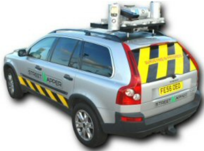
Figure 5.2: An example of the mobile mapping system [1].
