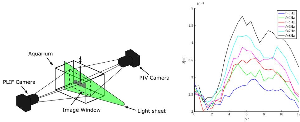
**Figure 1.** (left) Experimental setup scheme and (right) mean vertical size of the patch varying the frequency.
