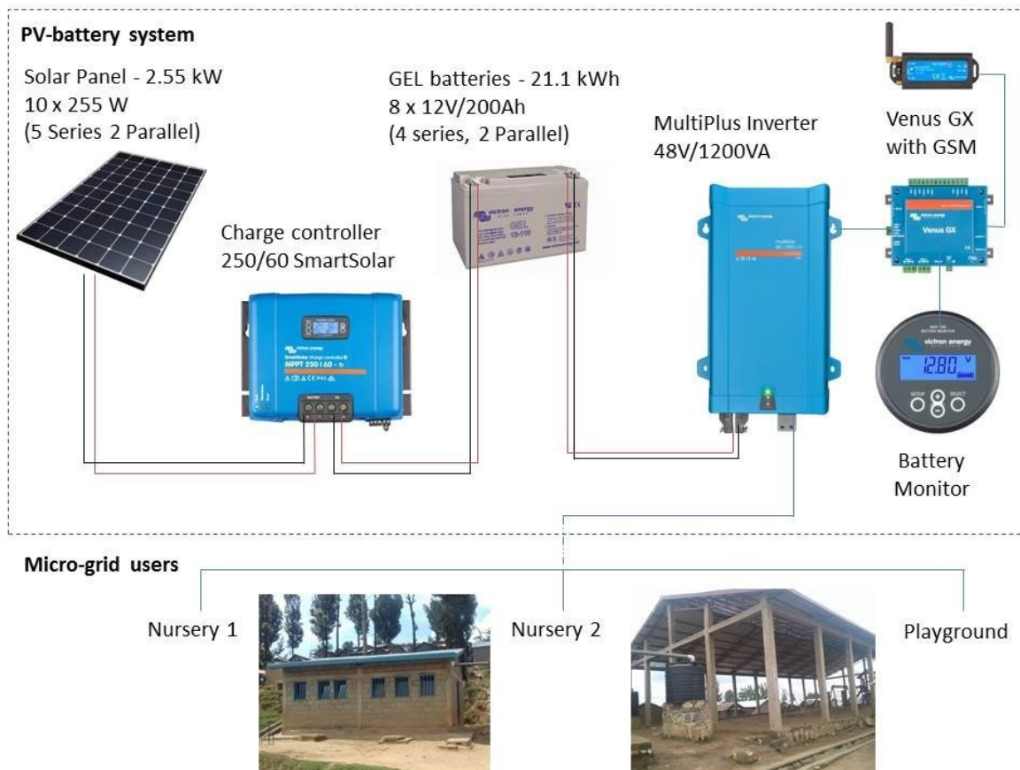
Figure 6.5: The micro-grid system components in the Kigeme refugee camp (HEED, 2020).
