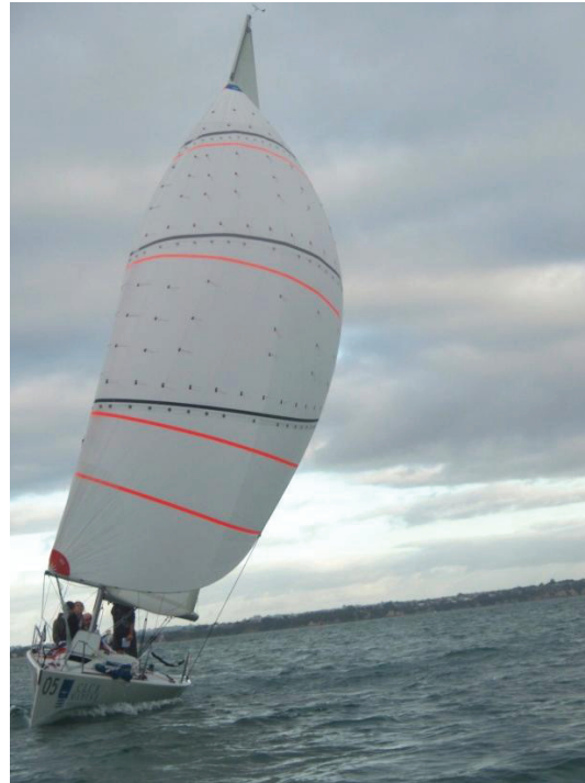
Figure 4: The yacht and the pressure-tapped sail. The black bands show the locations of the pressure taps.
