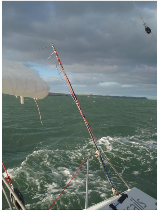
Figure 3: Pole supporting the Pitot-static probes (shown while sailing upwind after the tests).
