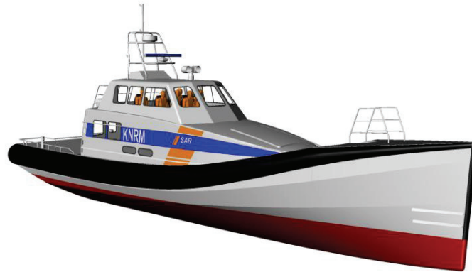
Figure 8 Proposal for a new SAR vessel for the KNRM with Loa = 21 m and V_s = 35 knots
