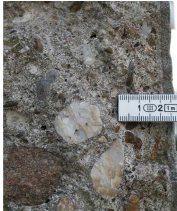
Picture of a concrete sample of the St Jobsveem, Rotterdam. A aggregate of gravel and different fractions can be seen. Which are not been graded well.
