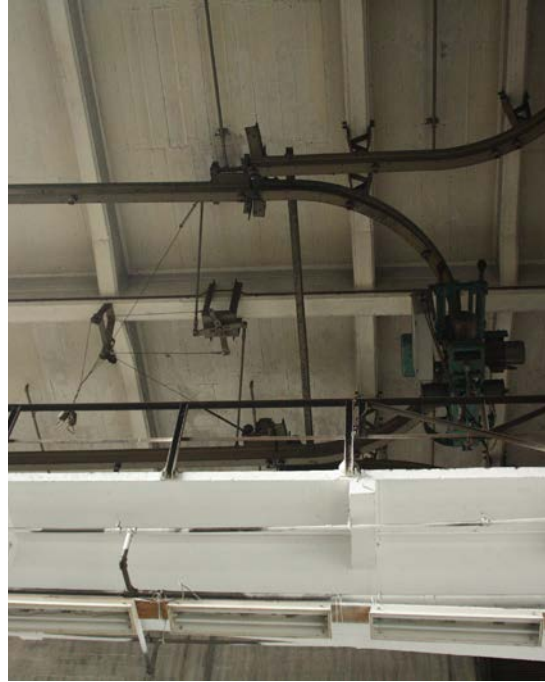
Image 2 - Rail changing system and operating cables
