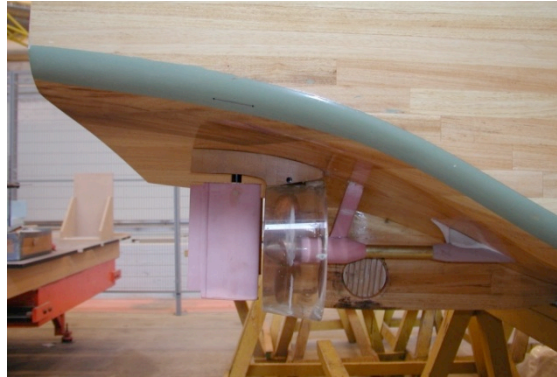
Fig 11: Buttock lines and propeller location.
