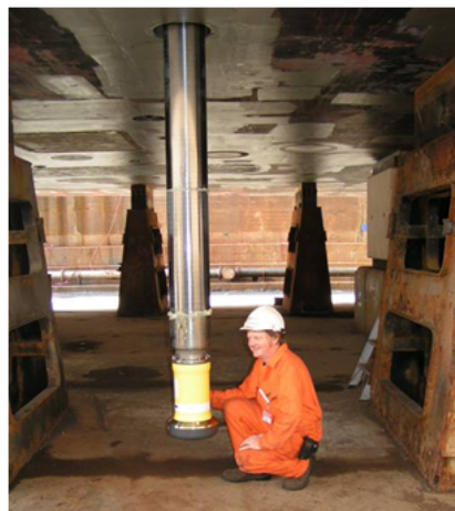
Figure 7 A through hull deployment machine
