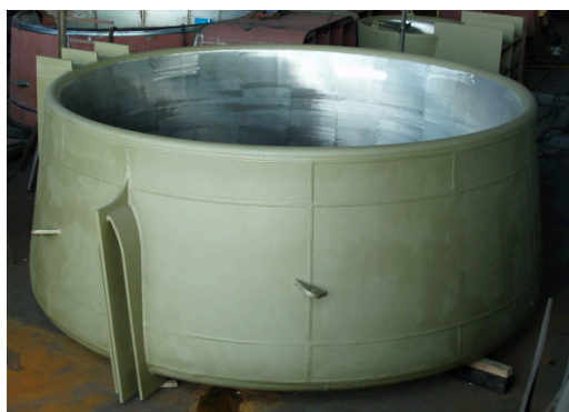
Fig 7: An AHT Ø4030 nozzle ready for dispatch. Leading edge of the nozzle is on the floor.
