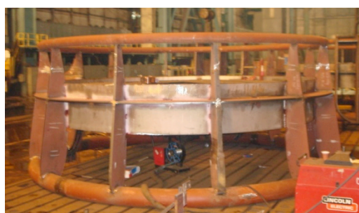
Fig 8: An AHT nozzle (ø4030) during assembly.
