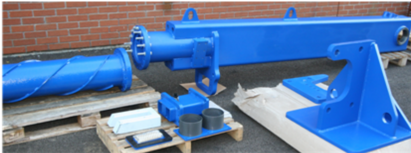
Figure 8 A Sonardyne over the side pole
