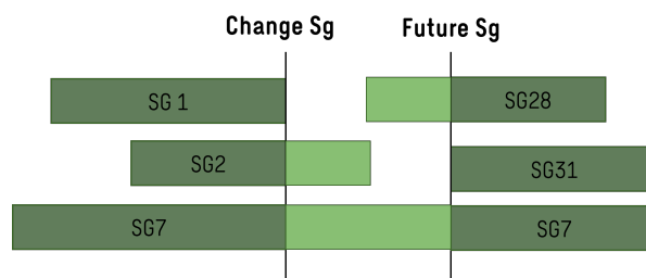
Figure 4.8: Heuristic intergreen maximisation, movement 1 has a conflict with cyclists movement 28 and both movements 1 and 2 conflict with pedestrians crossing in movement 31, Movement 7 is independent of all of them
