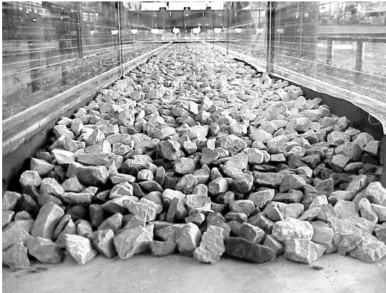
Figure 1.1: Left: laboratory model of a granular bed protection (present tests). Right: trial bed protection with 10-60 kg rock (Meulepas et al. , 1999).
