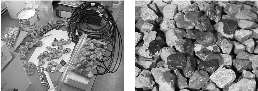
Figure 4.11: Left: mimicked bed under construction including moulds, wiring, epoxy-resin, etc. Right: mimicked bed in place, with target stone in the centre.
