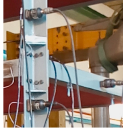
Fig. 2. Second instrumentation configuration for the energy flow analysis
