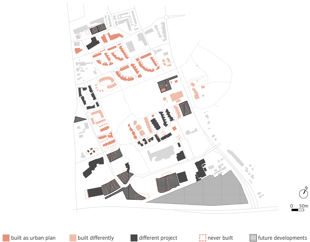
FIG. 3.3 Lanxmeer: urban plan, realisation, and future developments. Comparison between the original urban development plan (1997) and the current configuration (2025), highlighting the spatial evolution of the neighbourhood. The diagram distinguishes housing projects as initially planned, those realised to date, and proposed or recently initiated developments.
