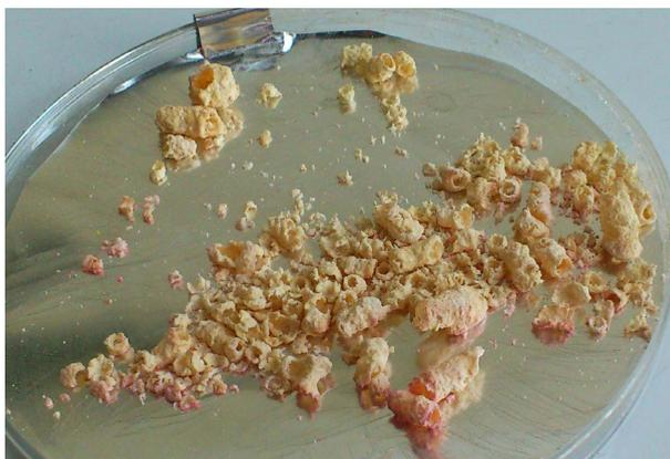
**Figure 5.4:** Example of material losses from an EC experiment using TNT and RDX in acetone
