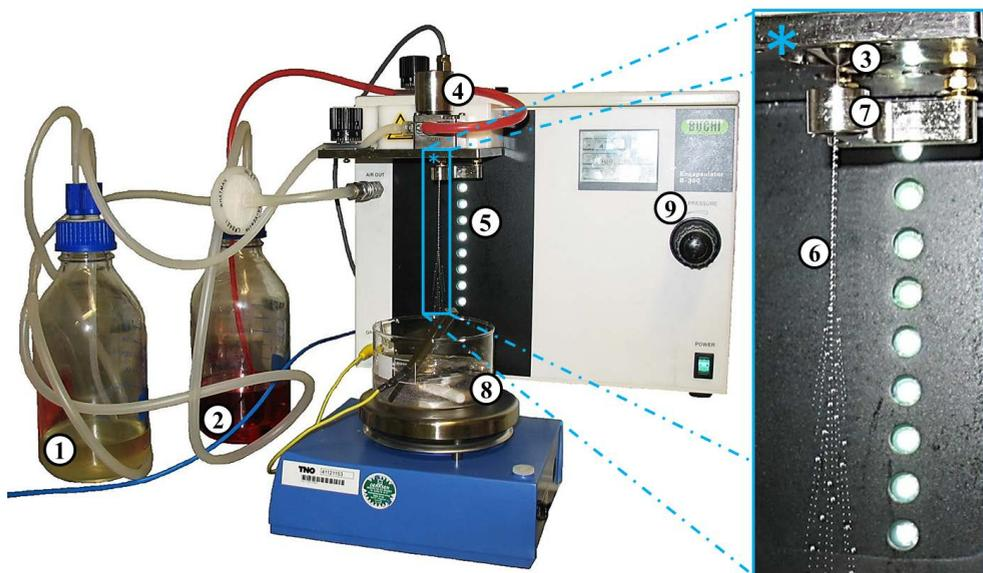
**Figure 6.1:** Büchi Encapsulator in core-shell configuration, with 1. Pressure bottle with immobilization mixture, 2. Pressure bottle with solution (red for illustration), 3. Concentric nozzle, 4. Vibration coil, 5. stroboscope for visualization, 6. Jet with droplets, 7. Electrostatic dispersion unit, 8. Cross-linking bath, 9. Controls.
