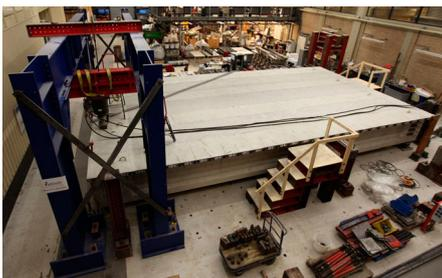
Fig. 4: The 1:2 scale model bridge deck in the laboratory (Photo: authors)
