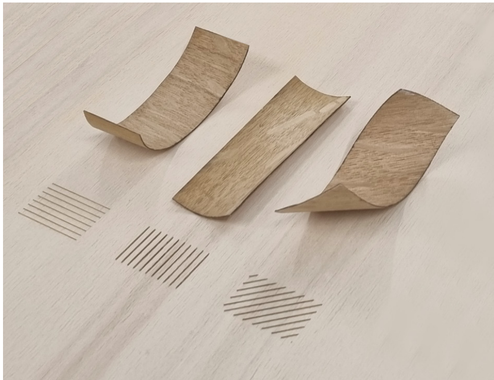
Fig 14. Samples tested with varying fiber orientations and their curvature result.
