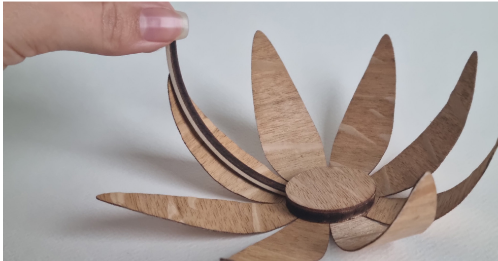
Fig 44. Method of measuring the curvature diameter. The figure shows the custom diameter gauge being held against a segment of the sample structure, measuring the exact curvature diameter.
