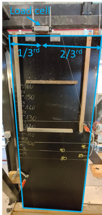
Figure 3.10: Assembly of load cell to the wood plate
