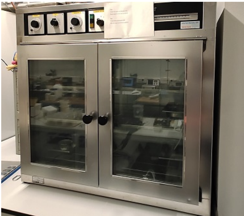
Figure 3.6: Samples kept in oven at temperature of 220^{\circ}\text{C}
