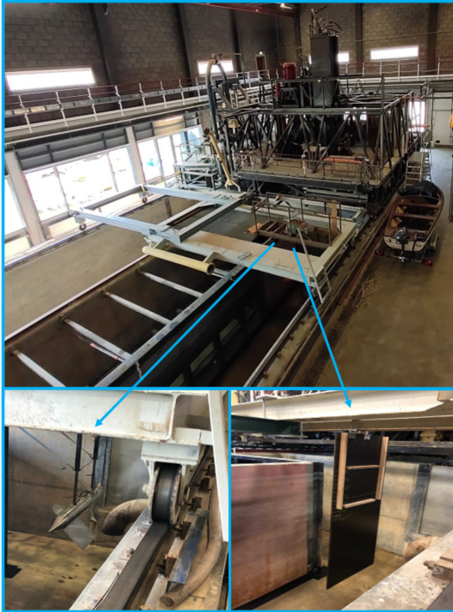
Figure 3.17: Location of the towing object in the test set-up
