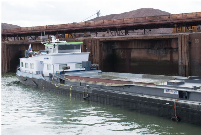
Figure 3.15: Water layer on top of hopper
