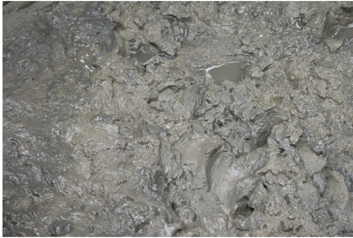
Figure 3.14: Mud lumps in hopper
