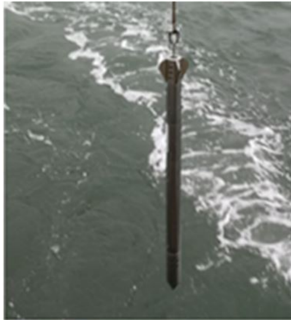
Figure 2.3: The image shows the Graviprobe device. Image taken from (Kirichek et al., 2020).
