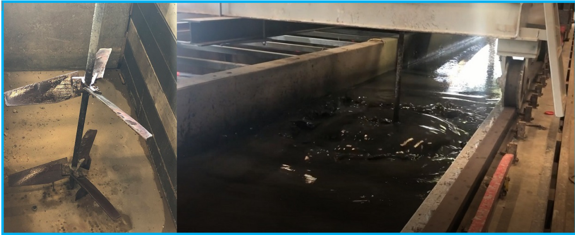
Figure 3.16: Blade rotor setup hanged to the frame to mix the fluid mud in flume.
