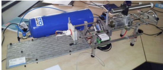
Figure 9 Test bench build by Smit to measure the Bowden cable displacement and the corresponding activation forces and pinch forces.
