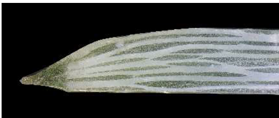
Fig. 8. Cross-section of the laminate after subsequent forming and reverse forming.
