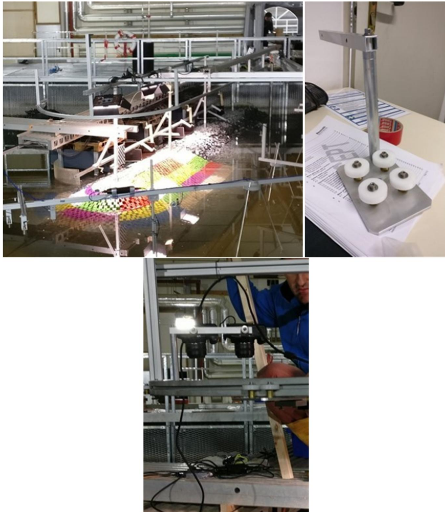
Figure 4. Left: rail to support the photographic cameras and the Kinect motion sensor; Middle: wagon to carry those cameras; Right: wagon on the rail with two cameras.
