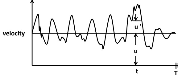
Figure 3.8: Variation of instantaneous velocity in time (van Rijn, 2008)
