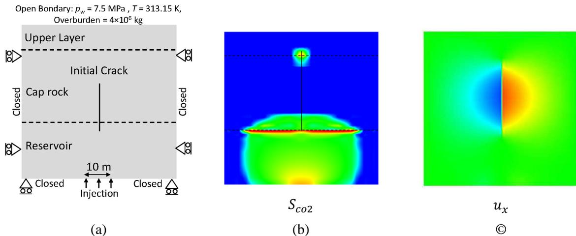
Fig.1 CO<sub>2</sub> geosequestration: (a) geometry and boundary conditions, (b) CO<sub>2</sub> saturation and (c) horizontal displacement.
