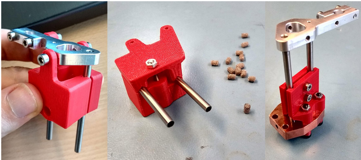
Figure 5.14: 3D printed brackets (red) as used to align the metal tubes to the top interface (left) and thruster body (right) during glueing. The metal foam pieces that were inserted into the pressure sensing tube are also shown (middle).
