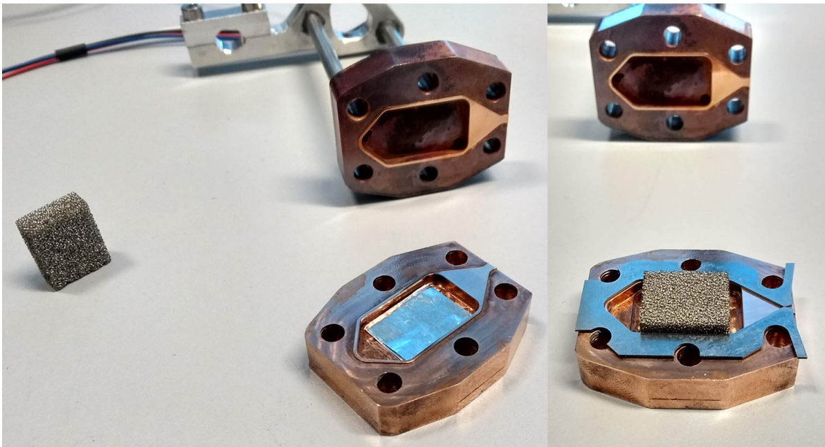
Figure 7.7: Re-polished copper blocks with aluminium foil spacer (left), nozzle profile, and metal foam (right) during assembly.
