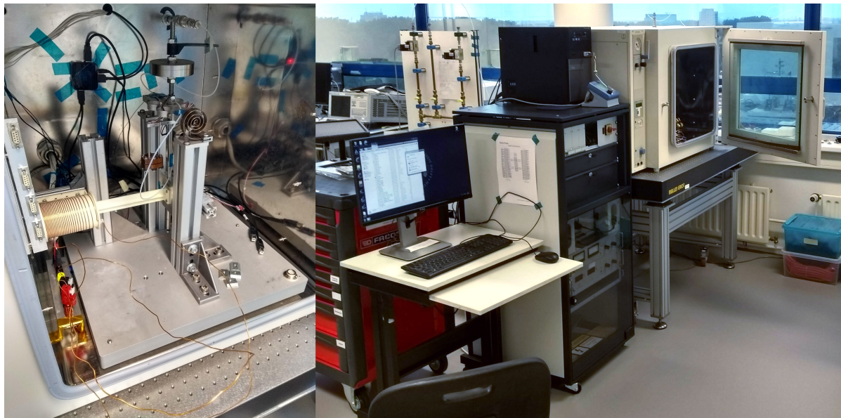
Figure 6.1: Overview of the thrust bench used for testing (left) and the equipment used to operate it in a vacuum (right).
