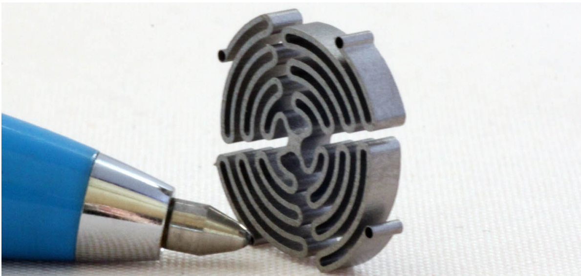
Figure 2.8: Component created with micro water-jet cutting by FinePart, ball-point pen for scale.
