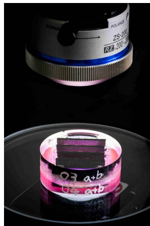
Figure 6. Embedded micrograph underneath optical microscope.
