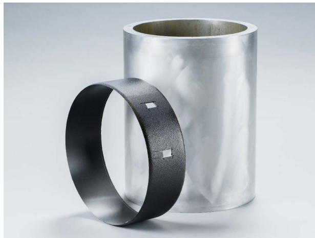
Figure 2. Tubular specimen ( \varnothing 350 mm) in front of aluminum mandrel.
