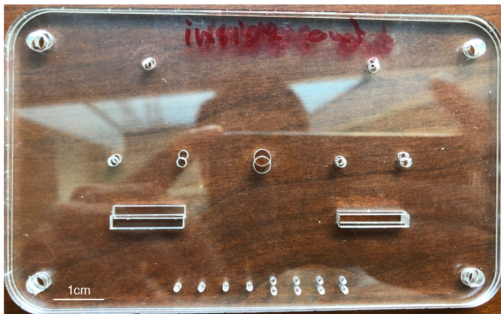
Figure C.4: Two sheets of PMMA cut from the same file with the same software settings. Variation in cut out locations can be observed. Some variations would be several millimeters, making correct alignment impossible.
