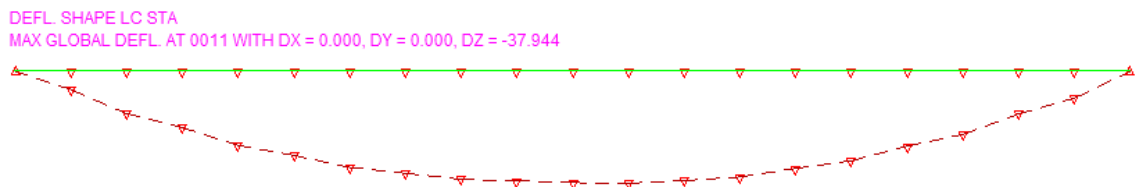
Figure G.4: Cable deflection along its length, loaded by self weight using 20 nodes in a linear static SACS analysis. Max deflection is -0.38 m.
