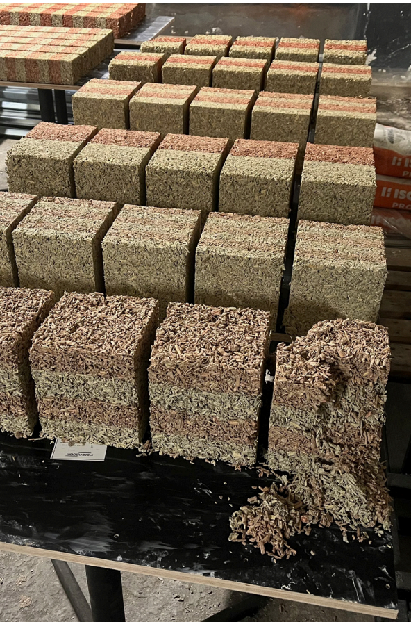
Fig 7.16 C min test: 10 % compaction, just enough initial bond
