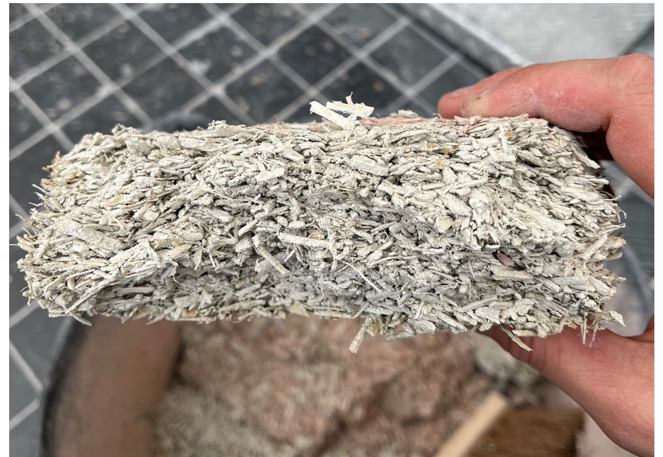
Fig 6.9 Cross section of compressed sample, torn by hand. The shivs are stacked horizontally, but the orientation of their long axes remain randomly distributed in the plane.
