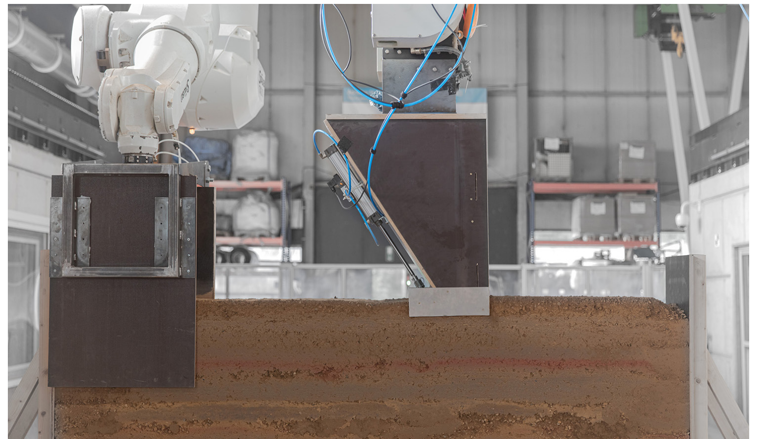
Fig 4.21 Fully CNC controlled material feeding and ramming by Kloft
