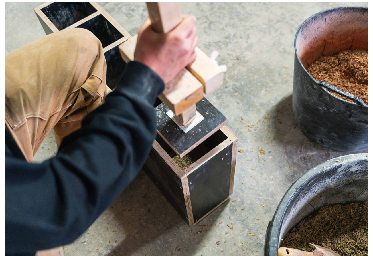
Fig 7.21 Compacting the material with the rammer until sliding clamp hits the rim of the mould
