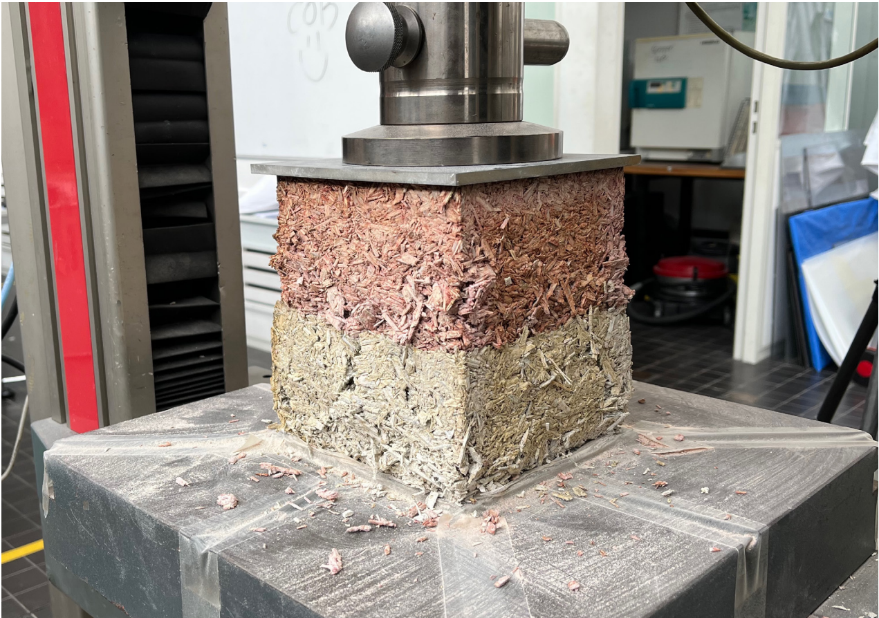
Fig 10.15 Failure at weakest link: lowest density region
