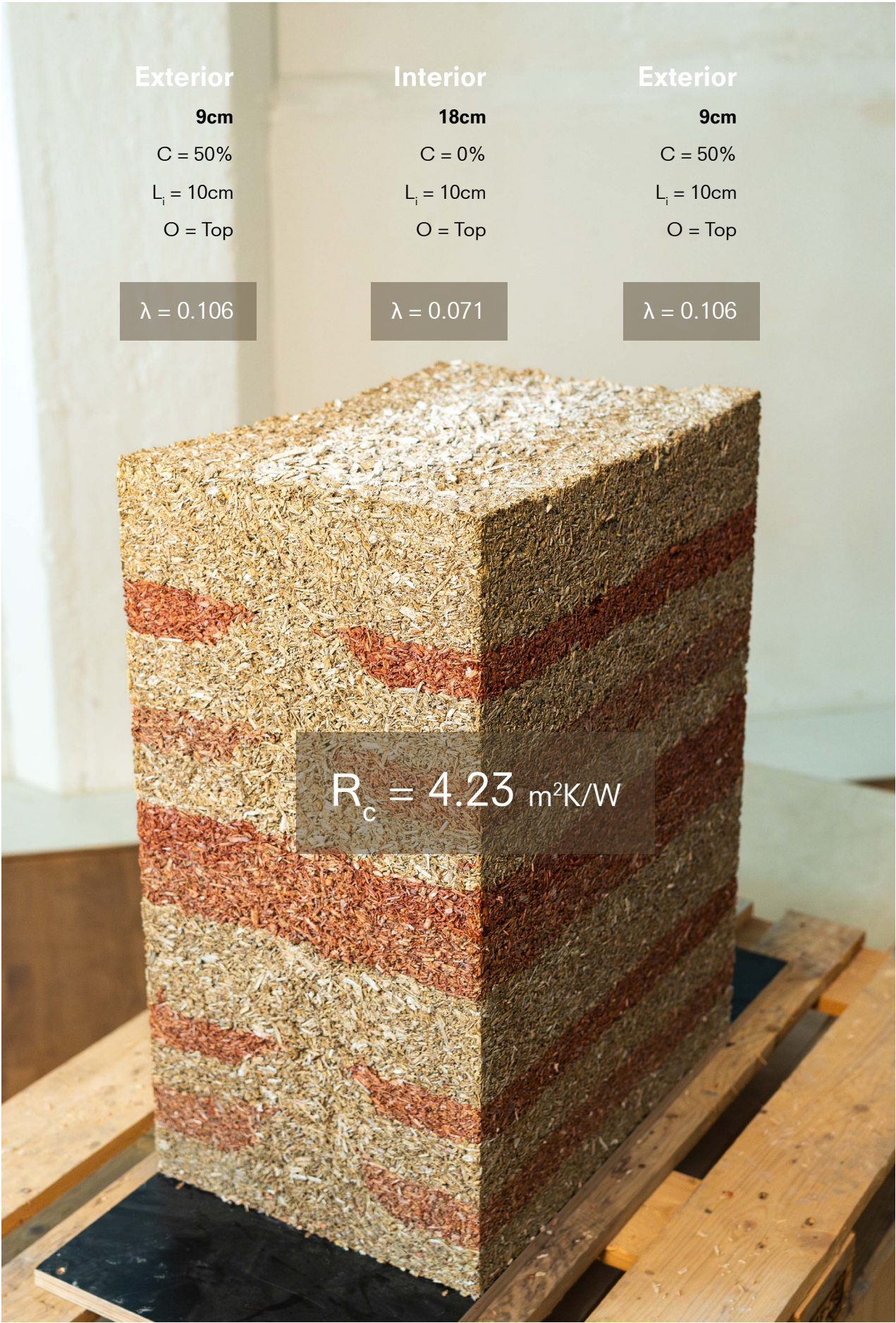
Fig 9.18 Measured thermal conductivities applied to 1:1 mockup wall.
