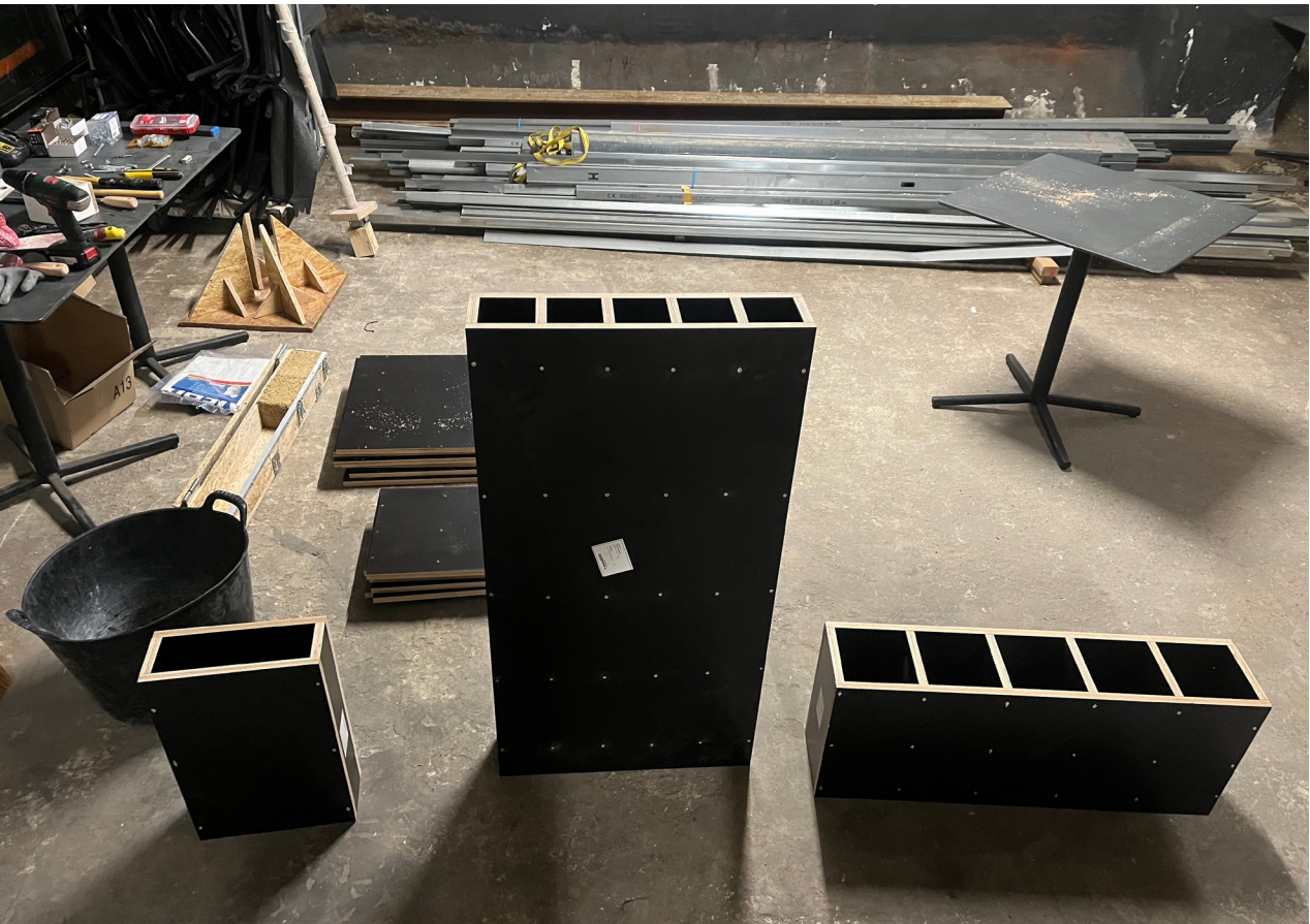
Fig 7.5 Betonplex moulds. LTR: Single panel mould, five-fold column mould and five-fold cube mould
