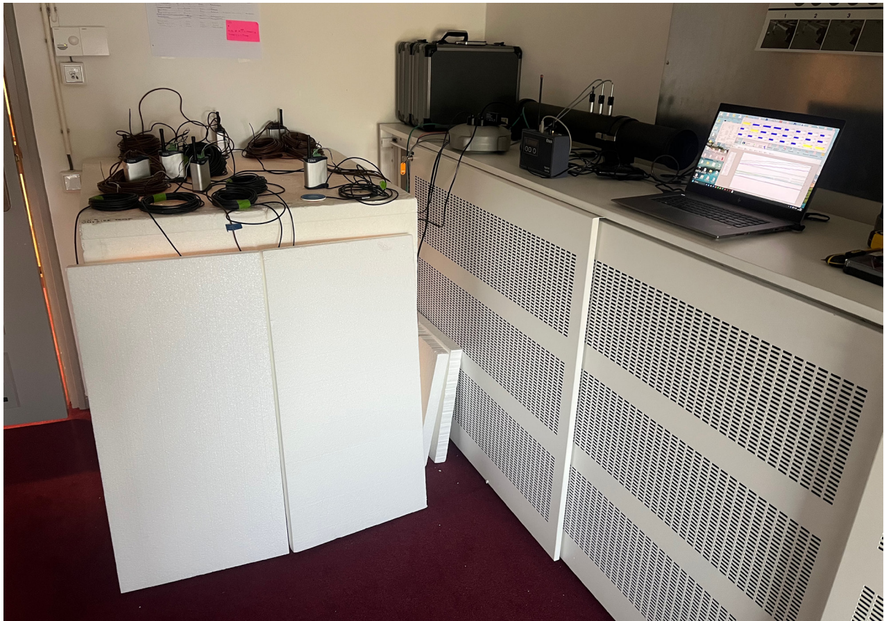
Fig 9.10 Setup during testing; EPS panels in front to prevent air stream, transmitters and dataloggers on top of the hotbox
