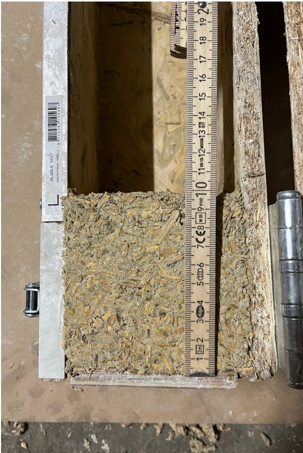
Fig 7.11 C max test for 5x initial layer height L_i = 5 cm
