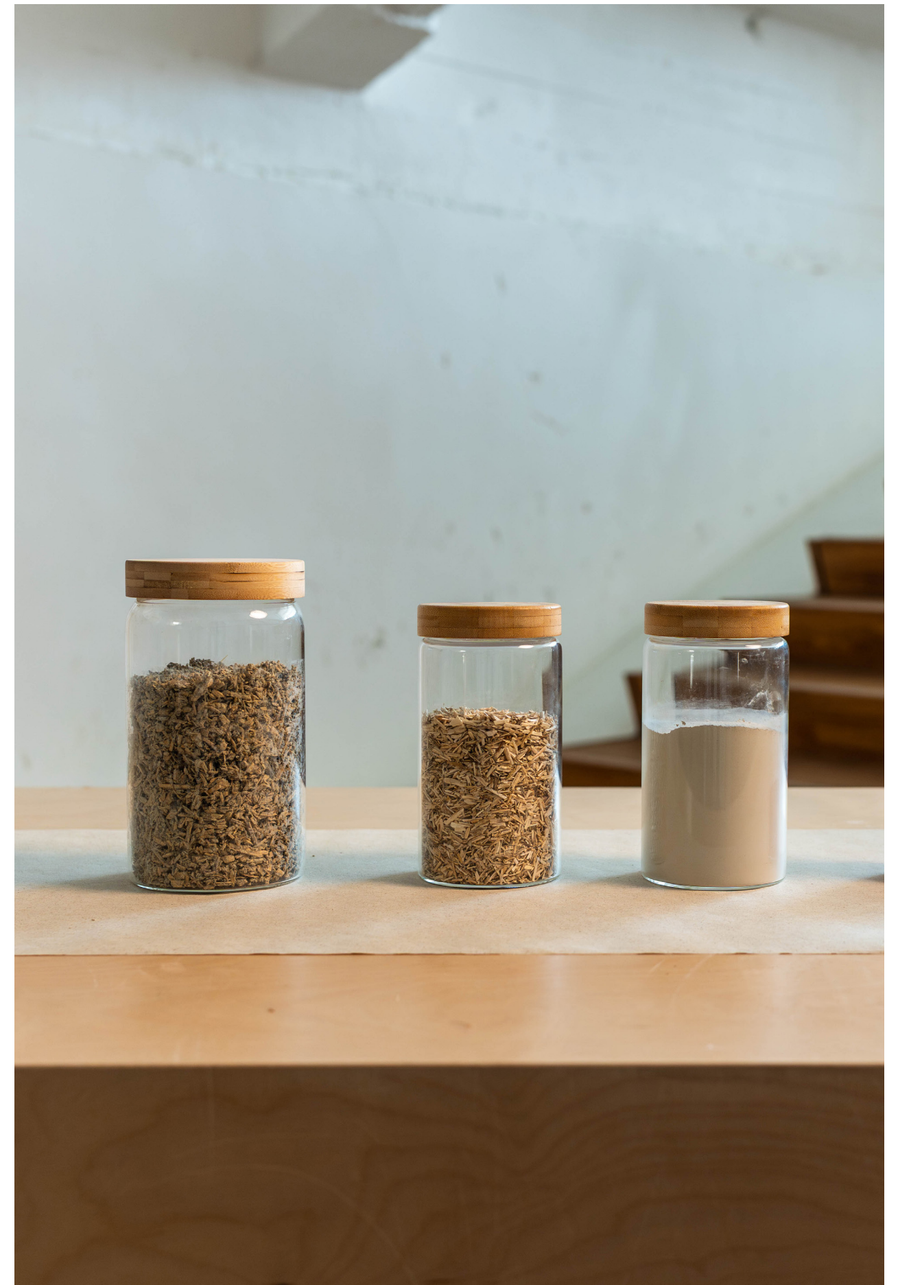
Fig 3.10 Hempcrete (left) and its components: hemp shivs (middle) and lime (right)
