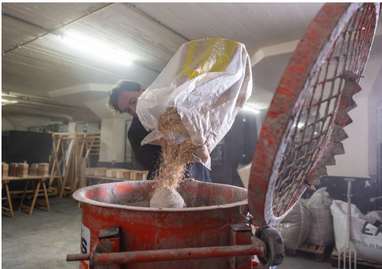
Fig 7.19 Adding the hemp shivs to the lime mixture in the 100 L pan mixer
