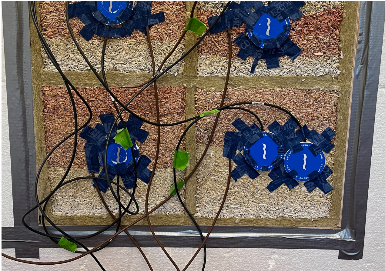
Fig 9.14 Left: Sensor in lowest density zone (A4). Richt: Sensors in interface zone (A5) and highest density zone (A5*)
