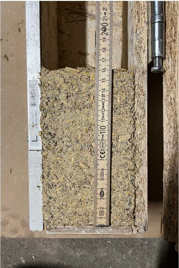
Fig 7.12 C max test for 4x initial layer height L_i = 10 cm
