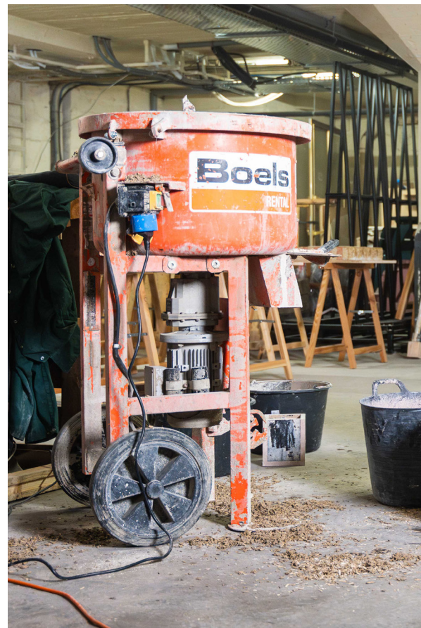
Fig 7.9 100 L electric pan mixer
