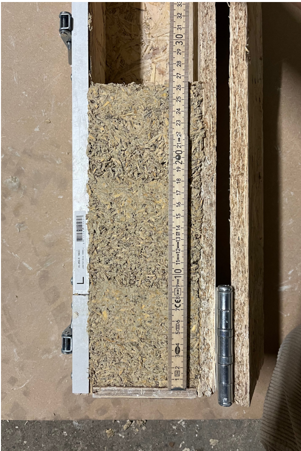
Fig 7.13 C max test for 3x initial layer height L_i = 20 cm
