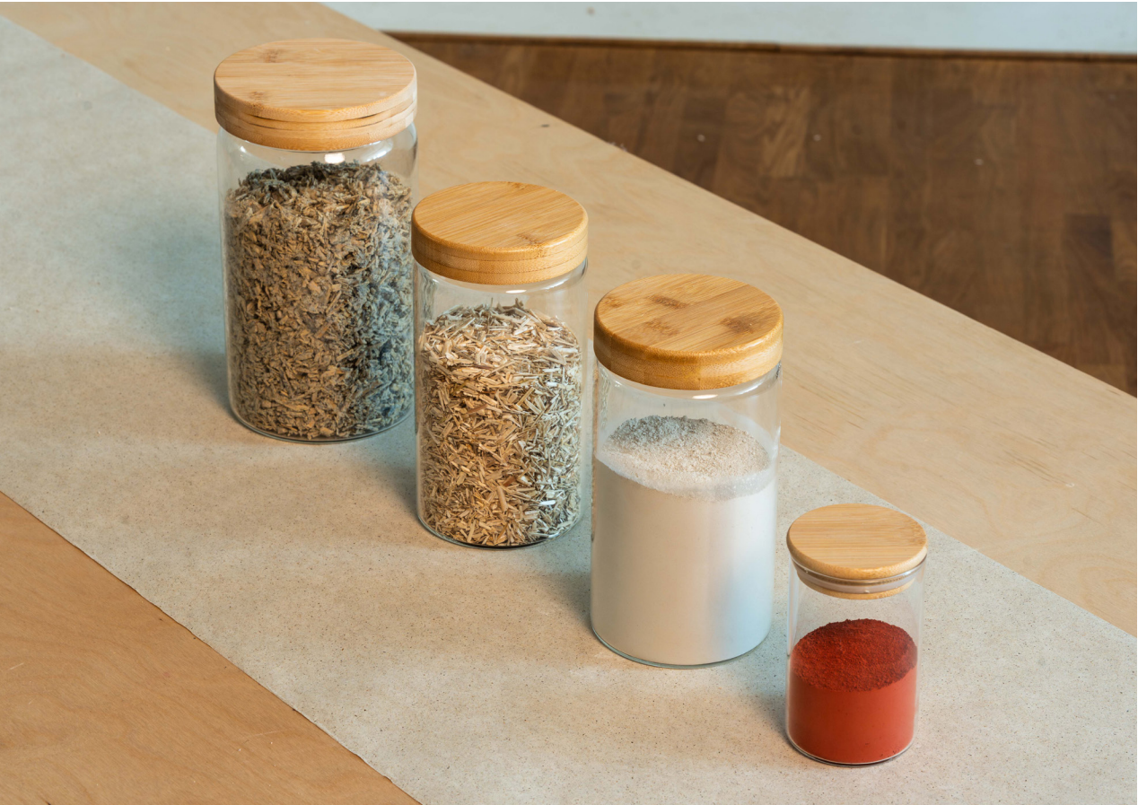
Fig 6.2 Used materials, LTR: EXIE CaNaCrete, Isohemp shivs, Prokalk Lime and natural clay-derived pigment “Rouge Venitien”
