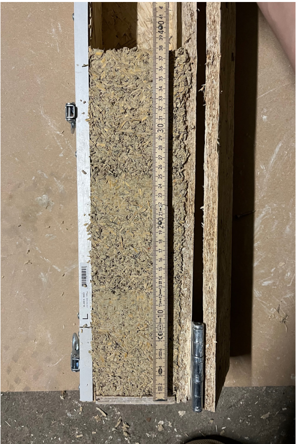
Fig 7.14 C max test for 3x initial layer height L_i = 30 cm
