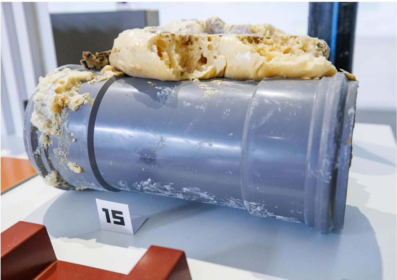
Fig 1.5 PVC pipe with PUR-foam insulation stuck to it
