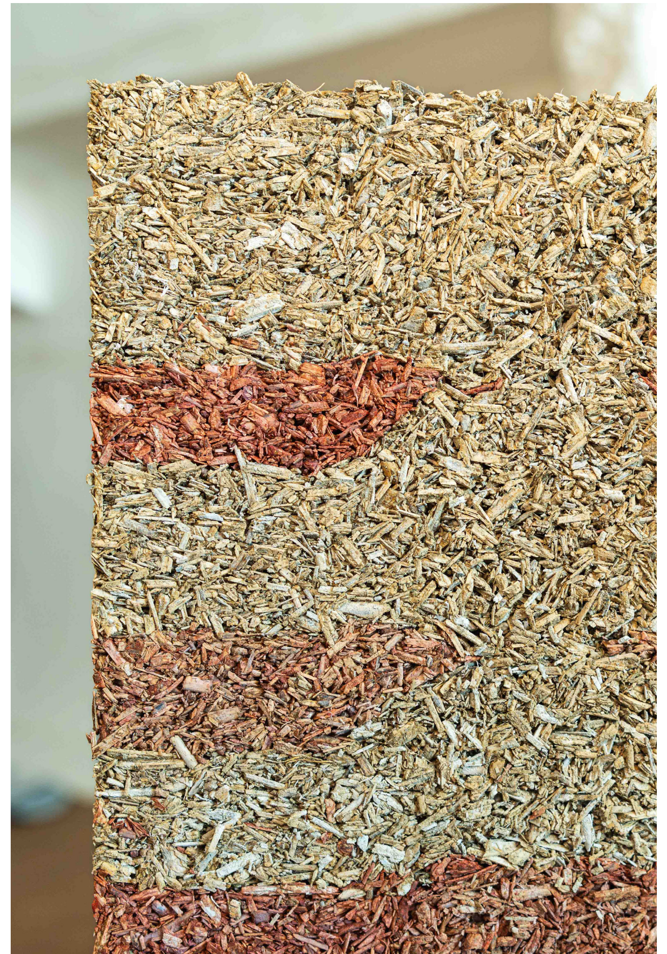
Fig 3.6 Left part: compacted hempcrete, shivs oriented flat, right part: uncompacted: shivs randomly oriented
