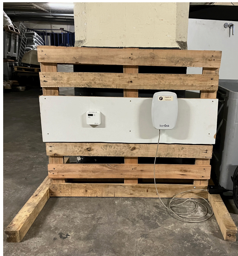
Fig 7.3 'Weather station' with FL Fresh datalogger (left) and Kerlink gateway (right)
