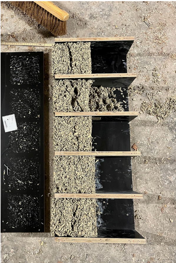
Fig 7.15 C min test: 0 % compaction, no sufficient initial bond
