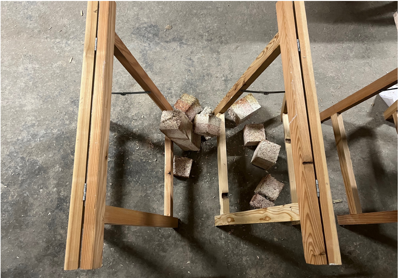
Fig 11.3 Sample failed at the layer interfaces
