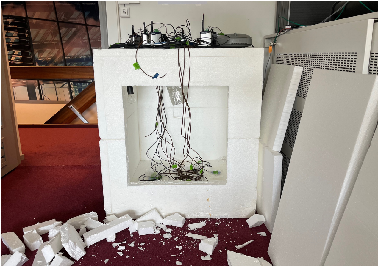
Fig 9.8 Hotbox after cutting out the opening
