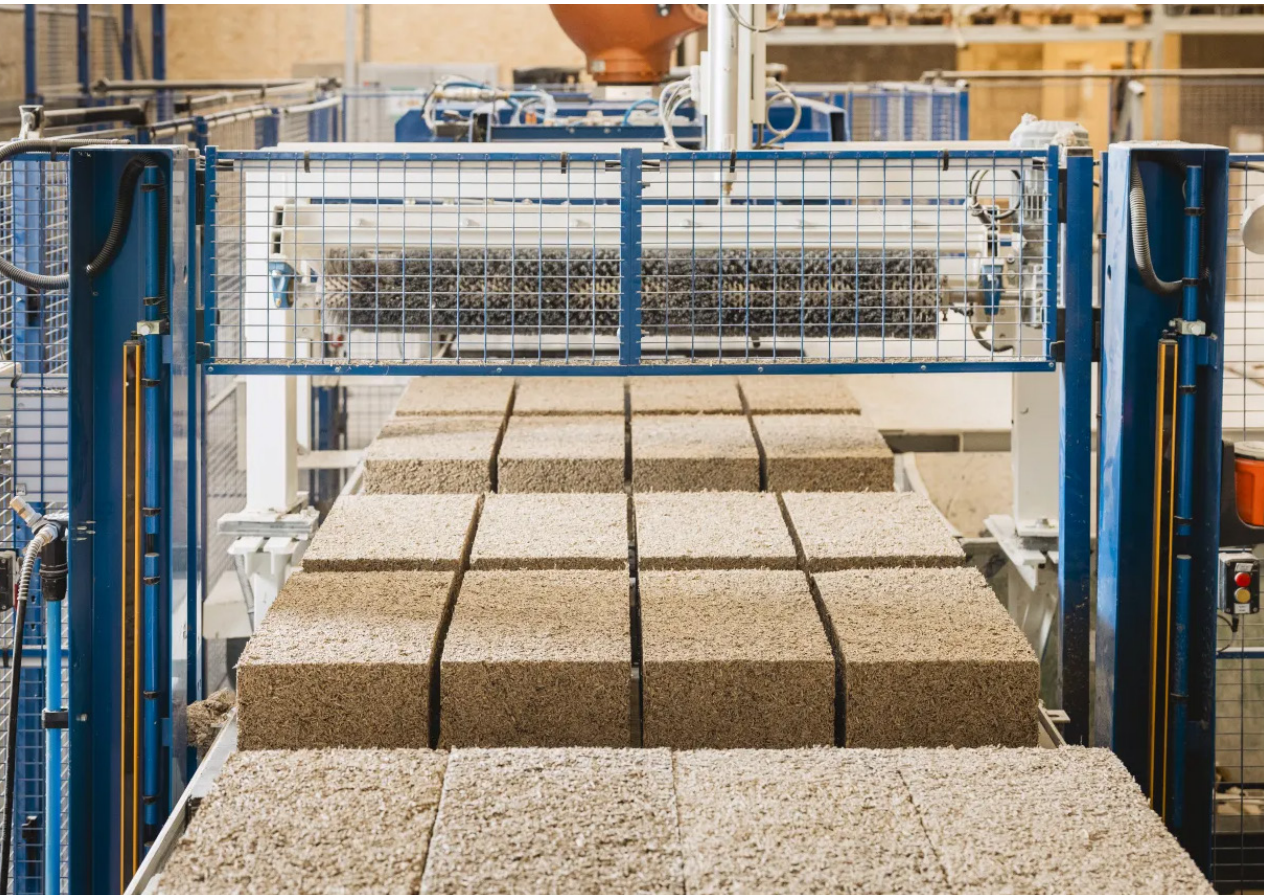
Fig 4.10 IsoHemp's hempcrete blocks at their factory in Fernelmont, Belgium
