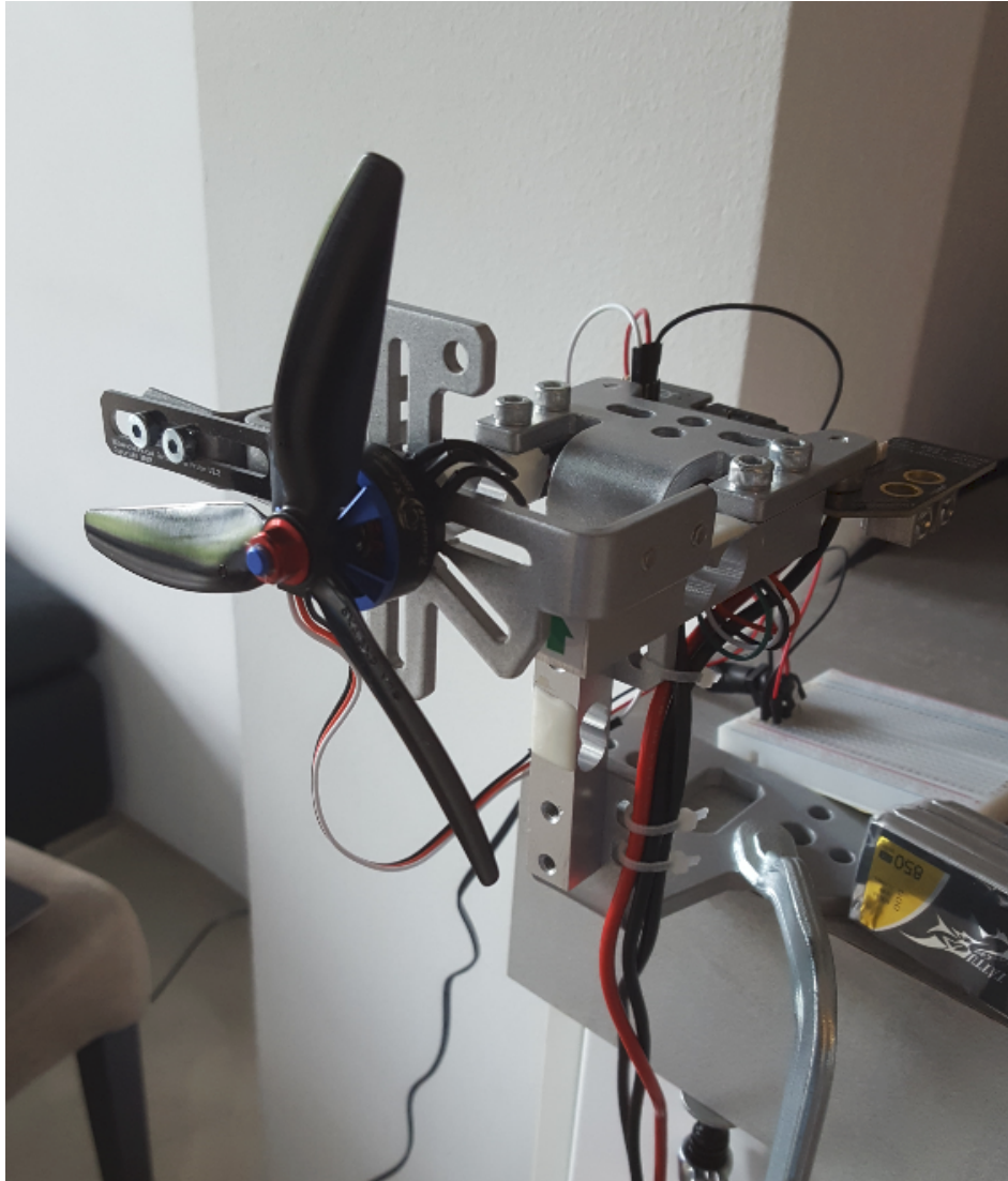
Figure 6-5: Motor testbench to collect data for system identification.
