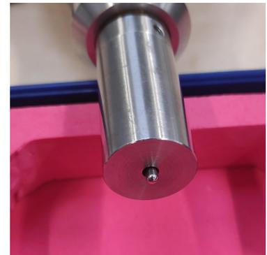
Figure 3.7: Tip of the shore hardness tester.
