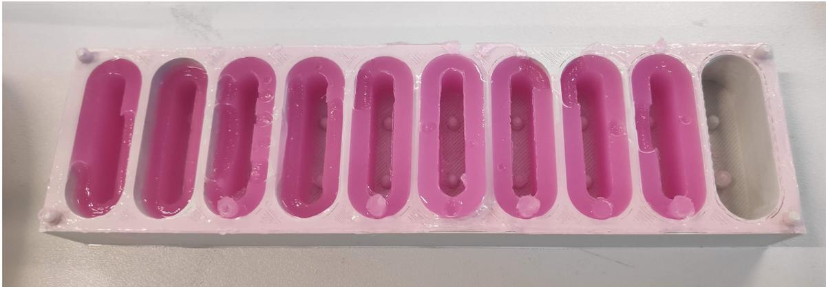
Figure E.2: Air defects influencing the shape of tensile sample of type 1.
