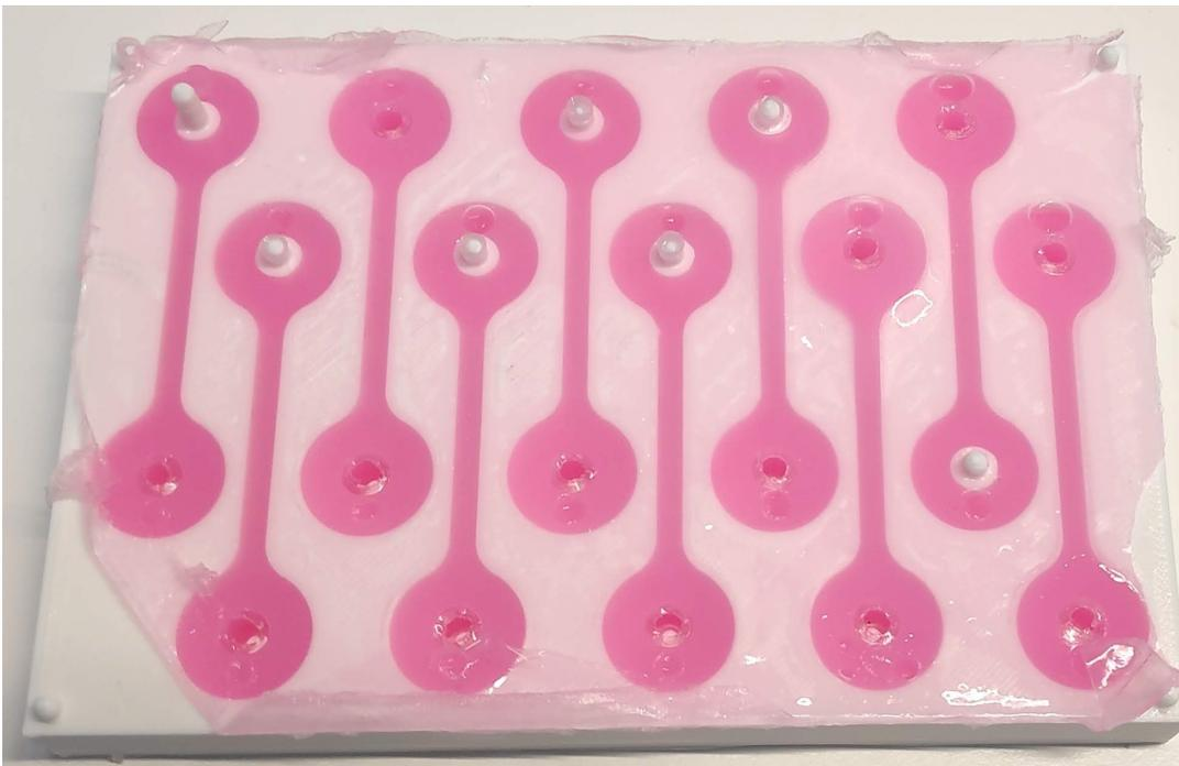
Figure E.4: Mould for the manufacturing of samples of type 2.
