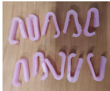
Figure 2.13: Failure point of type 1 samples
