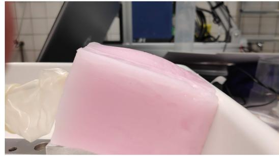
Figure 6.3: Overfilling of the PVA-phantom, during the experiment using the probe cover.
