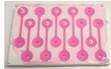
Figure 2.3: Mould with samples of sample type 2 prior to demoulding.
