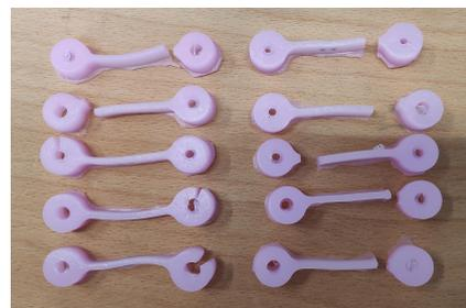
Figure 2.14: Failure point of type 2 samples
