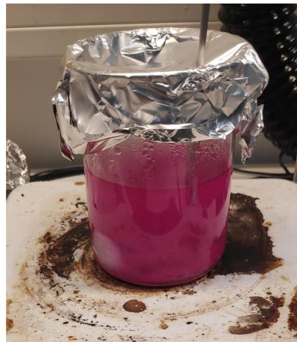
Figure C.1: Production of PVA-hydrogel, pink color is due to the used cooling liquid.
