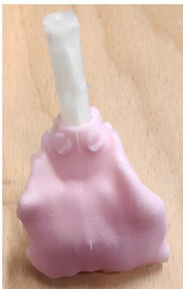
Figure 5.4: Insert with vaginal wall after de-molding.
