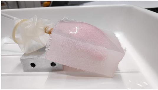
Figure 6.2: Overfilling of the silicone phantom, during the experiment using the probe cover.
