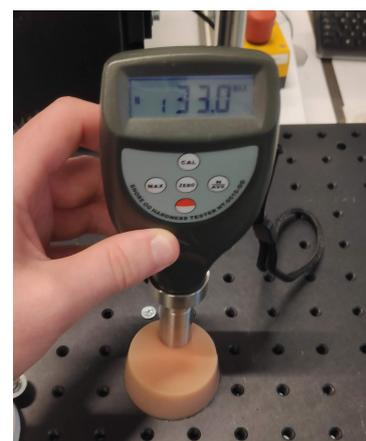
Figure 3.2: Indentation test
