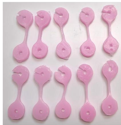
Figure 2.15: Failure point of type 3 samples
