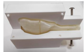
Figure 5.2: 3D-printed insert inside the mold for the vaginal wall.
