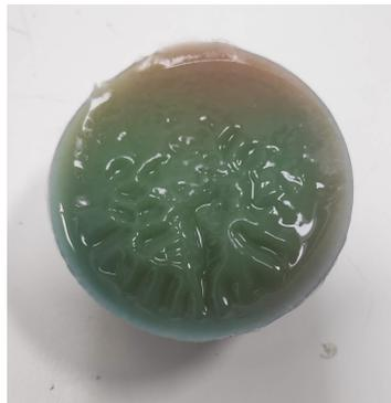
Figure 3.6: Rough surface of a PVA-hydrogel sample, this requires the samples to be tested upside-down
