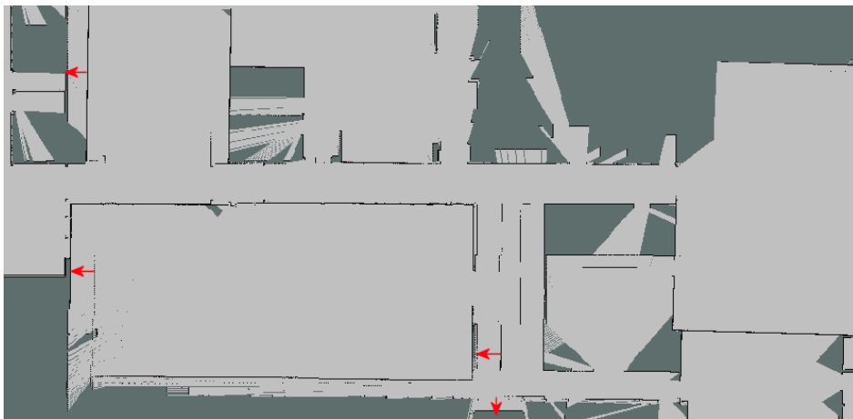
Figure 5-23: A partial map created by GMapping, the local environment in Figure 5-22. The loop closure offsets are visualized with red arrows.
