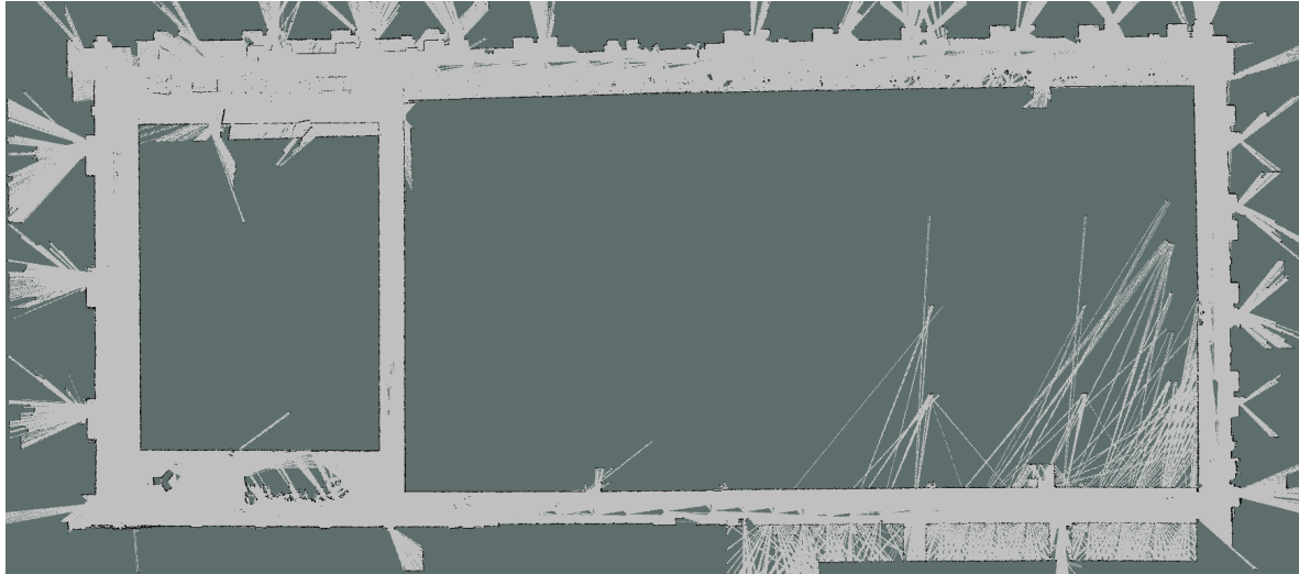
Figure 5-11: GMapping in experiment 2, unsuccessful loop closure.
