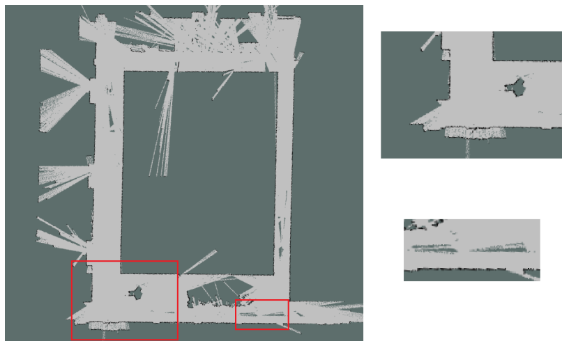
Figure 5-6: A map of the small loop at IDE created by GMapping with standard parameters. Red rectangles indicate the areas of the close-ups which are visualized on the right.
