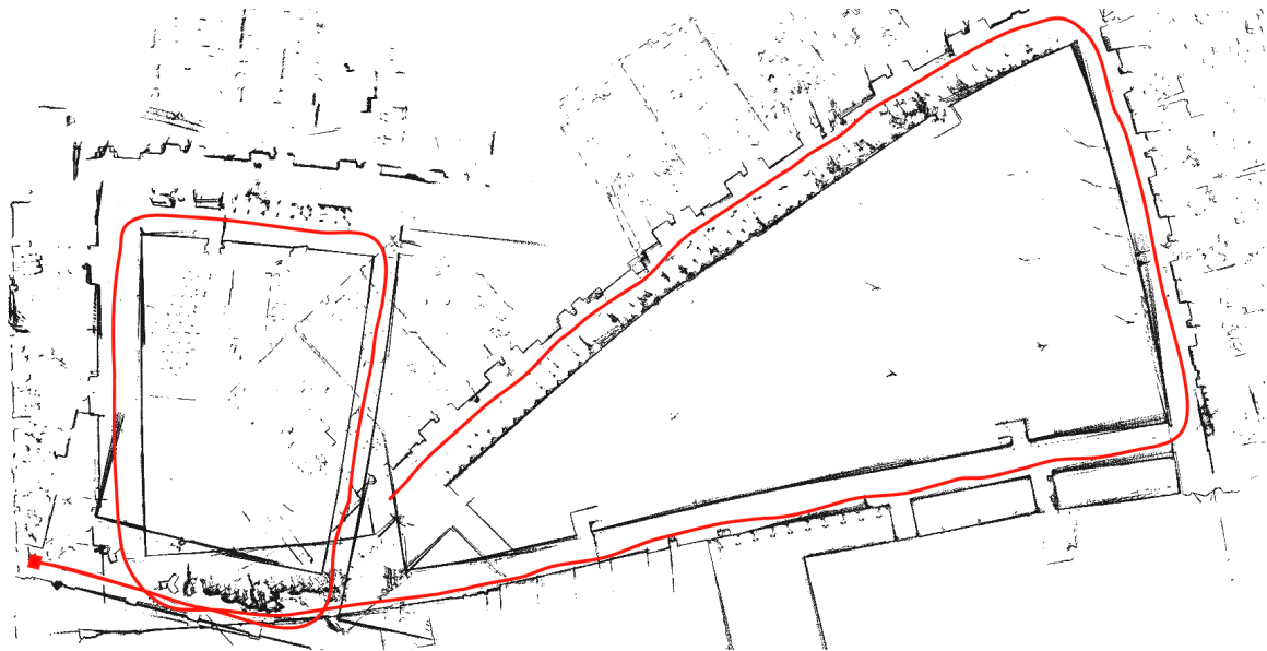
Figure 5-10: A raw point map of the small and large loop at IDE. Constructed from laser point projection from pure odometry. The trajectory is shown in red with a square at the start point.
