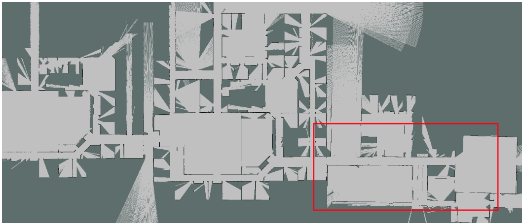
Figure 5-22: A GMapping created map of the simulated environment in experiment 3. The close up of Figure 5-23 is located in the red rectangle
