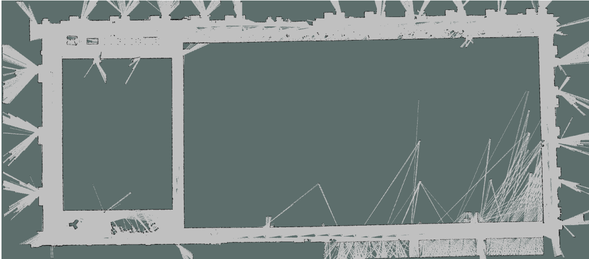
Figure 5-13: GMapping in experiment 2, successful loop closure
