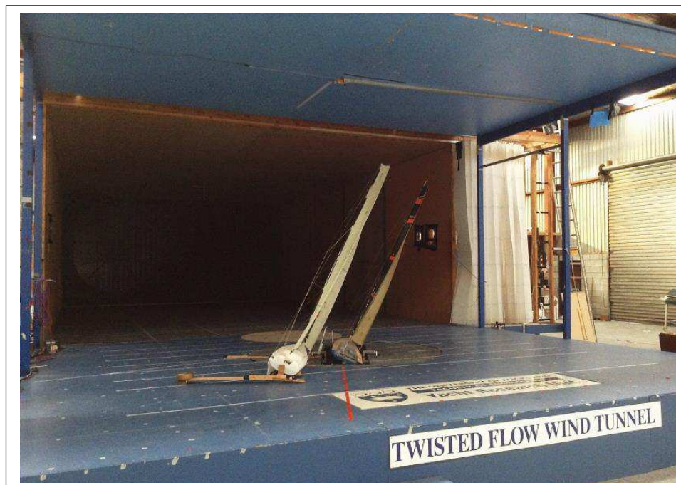
Figure 1 Two boat testing in the University of Auckland Twisted Flow Wind Tunnel
