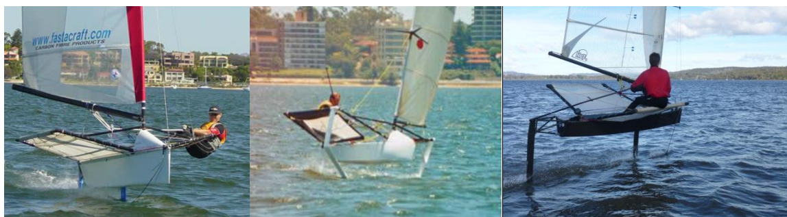
Figure 1 Fully-Submerged Foil Configurations (Left), Surface Piercing design (Middle), (Stevenson et al., 2004). Un-flapped foil sailed by the author (Right).
