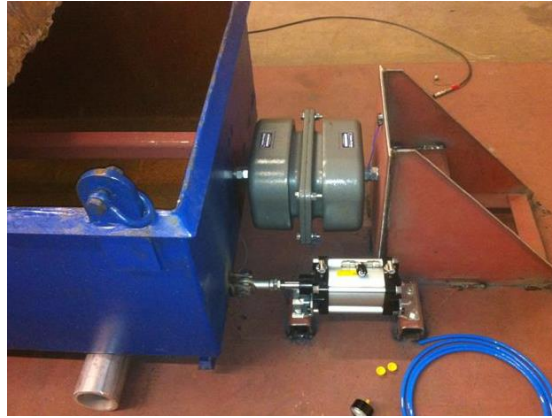
Figure 14 TMD, one of the four spring assemblies and damper
