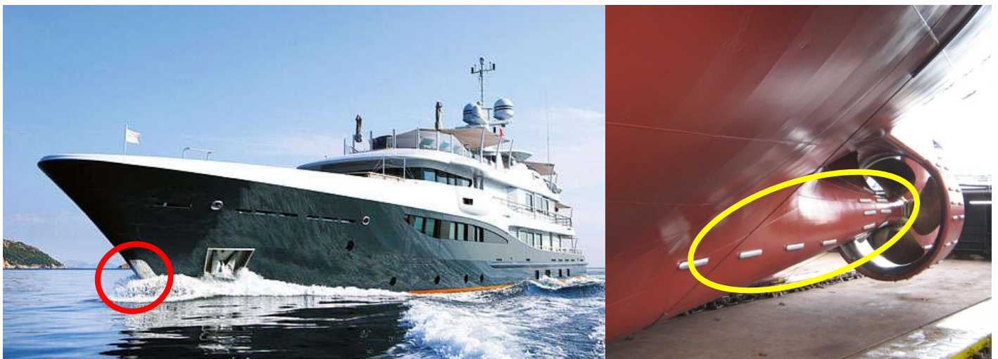
Figure 2: cases that were studied: left, stainless steel bow plate (source: Amels); right, composite streamline fairing bonded to steel or aluminum hull
