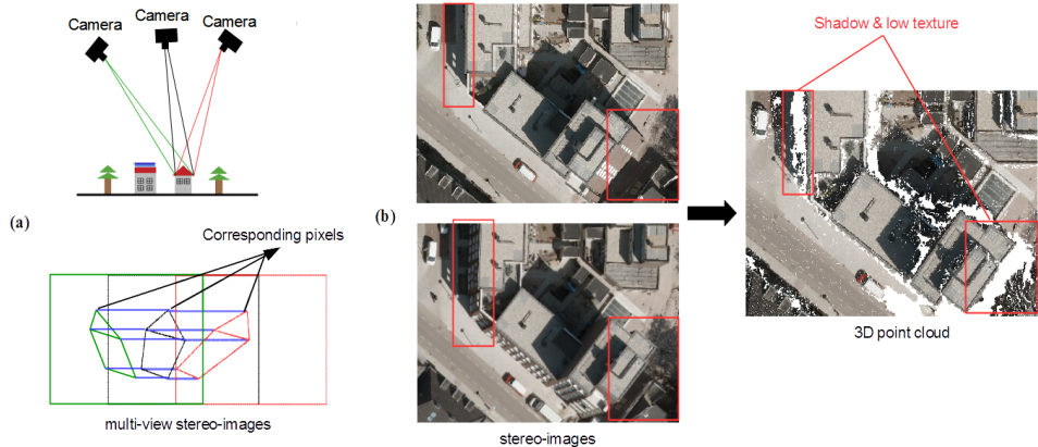
Figure 1.2: (a) Airborne cameras acquire stereo images showing the same 3D object in different positions. 3D point clouds can be extracted by finding corresponding pixels from stereo images. (b) 3D point cloud with color information extracted from VHR multi-view images. Two images from multi-view images are presented. In the red boxes, the quality of 3D point clouds is affected by shadow and low textures in the images.
