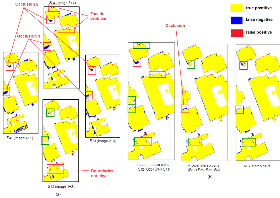
Figure 5.10: Visualization of extracted building areas, compared to reference data, for different scenarios. (a) the comparative building extraction results of integration with 4 individual stereo pairs from upper four images as shown in Figure 5.9b. The comparative building extraction results of integration with 4 upper stereo pairs, 4 lower stereo pairs and all 7 stereo pairs respectively as shown in Figure 5.9c. Red boxes show the problems which affects the accuracy of buildings, while the green boxes show the problems have been resolved by integrating multiple stereo pairs.
