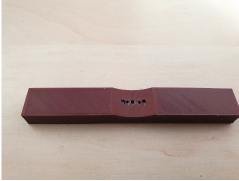
(a) The finger plate with drilled holes. The holes don't have the required accuracy since they are drilled manually.
