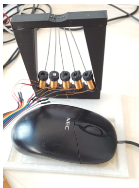
Figure 4.13: HTD prototype with a computer mouse built into the base, used as motion detection system for the dynamics
