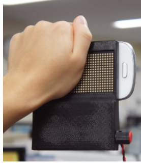
Figure 3.2: Example usage of an electro-tactile display (HamsaTouch), by Kajimoto [11]
