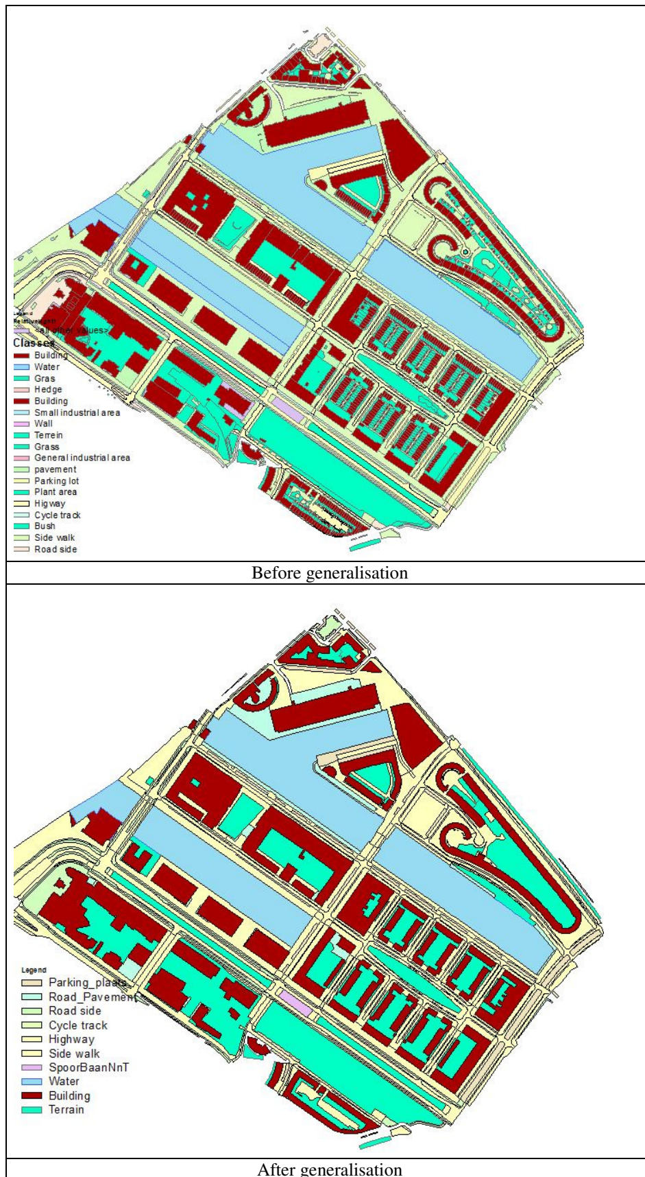
Figure 5: Results of automated generalisation of 1:10k dataset (below) from municipal data at scale 1:1k (left) in test area of Rotterdam.
