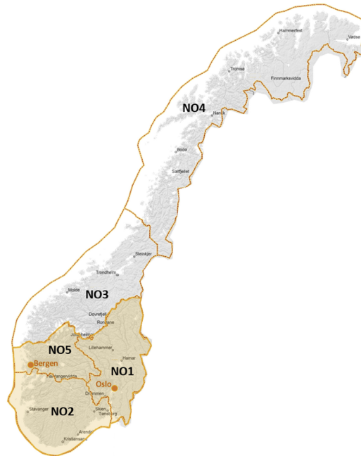
Figure 2.7: The five bidding areas of Norway. The southern part of Norway is highlighted in orange, where electricity prices increased following the European energy crisis. Reprinted from Hofmann and Lindberg (2024b)
