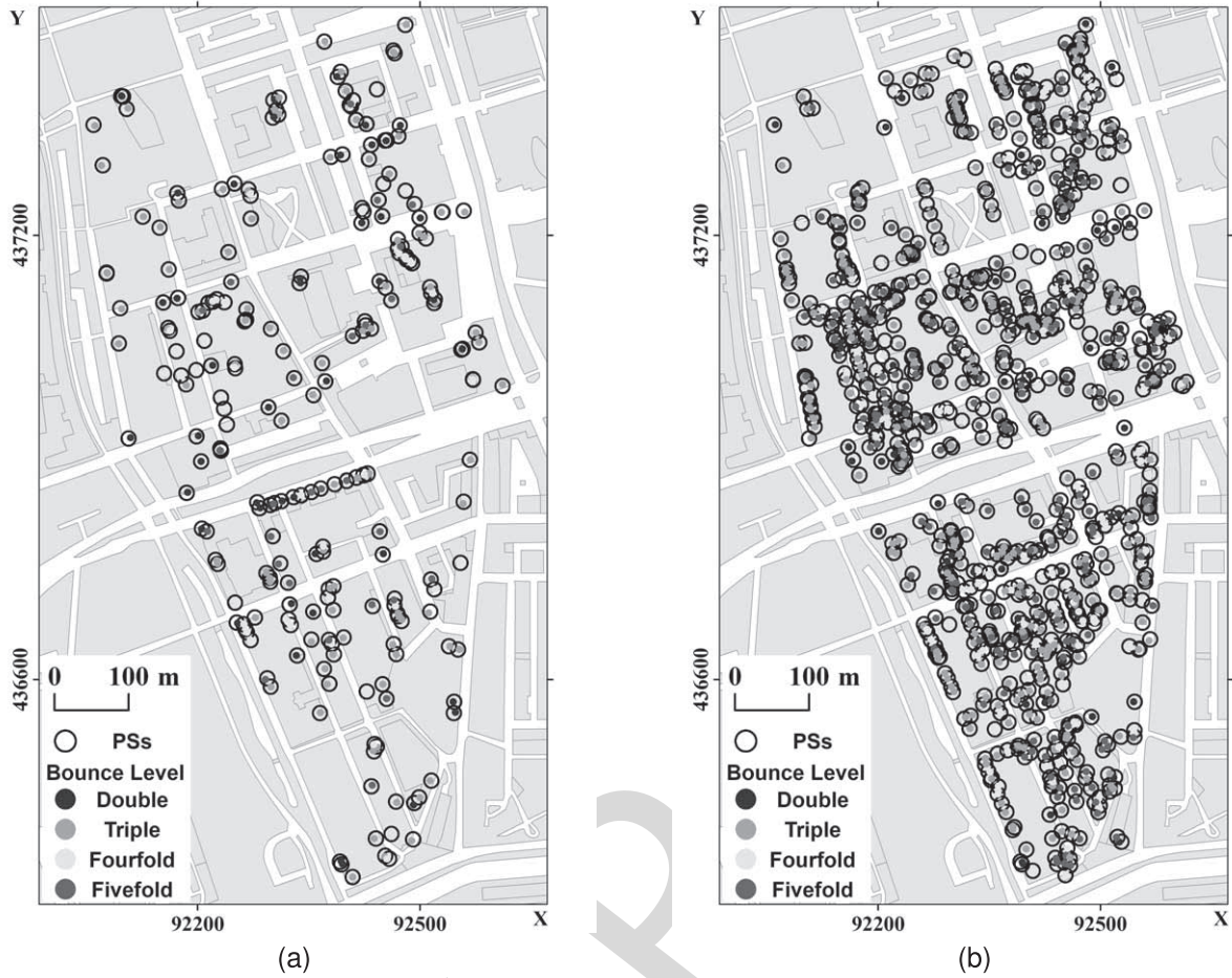
Fig. 11. Correspondence between SPs, shown as solid circles color-coded by bounce level, and matched PSs, shown as empty circles. (a) Left and (b) right correspond to simulations using the LOD1 and LOD2 models, respectively.
