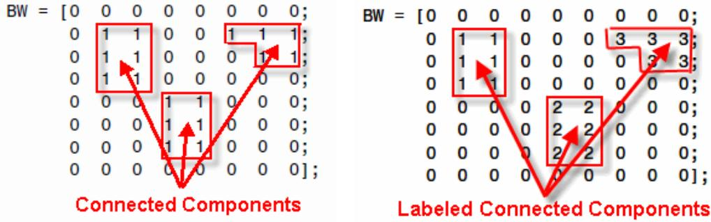
**Figure 5.1:** Figure showing how components are connected in a binary image. Obtained from the official MATLAB documentation [The MathWorks \[2018\]](#)
