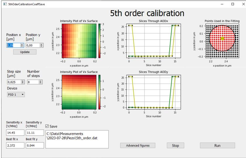
Figure 2.5: **Position calibration.** The bead was moved  $0.025\ \mu\text{m}$  per step, for 8 steps in each direction ( $\pm x$ -axis and  $\pm y$ -axis). The colors indicate the magnitude of the voltage with red positive voltages and blue negative voltages.
