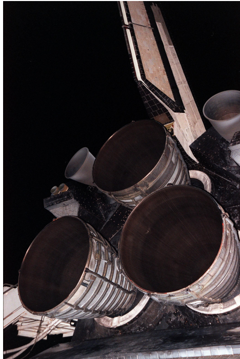
Figure 1.1: TOP contoured nozzles of the Space Shuttle Columbia's three RS-25s engines, following the landing of STS-93 (Courtesy: NASA)
